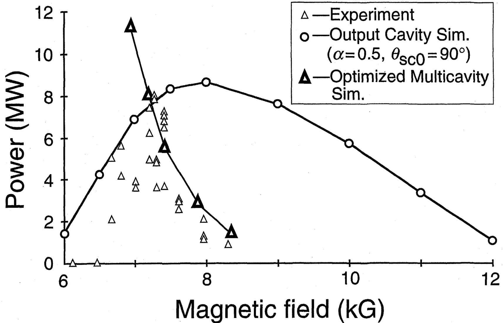
Figure 4. Measured output power versus magnetic field, compared with predictions of theory. Small triangles are data from single experimental shots. Circles are results from a time-dependent output cavity simulation assuming  $\alpha=0.5$  and  $\theta_{sc0}=90^\circ$ . Large triangles are the results from an optimized multicavity steady-state magnicon simulation.
