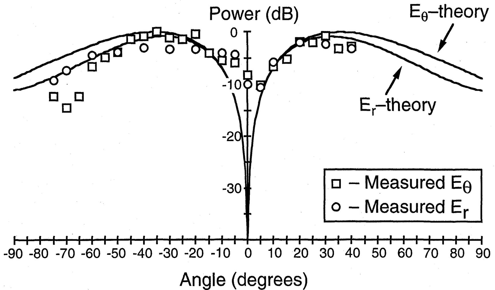
Figure 3. Measured far-field antenna pattern from 3.5-cm-diam. output compared to predictions of theory for the TE<sub>21</sub> mode.
