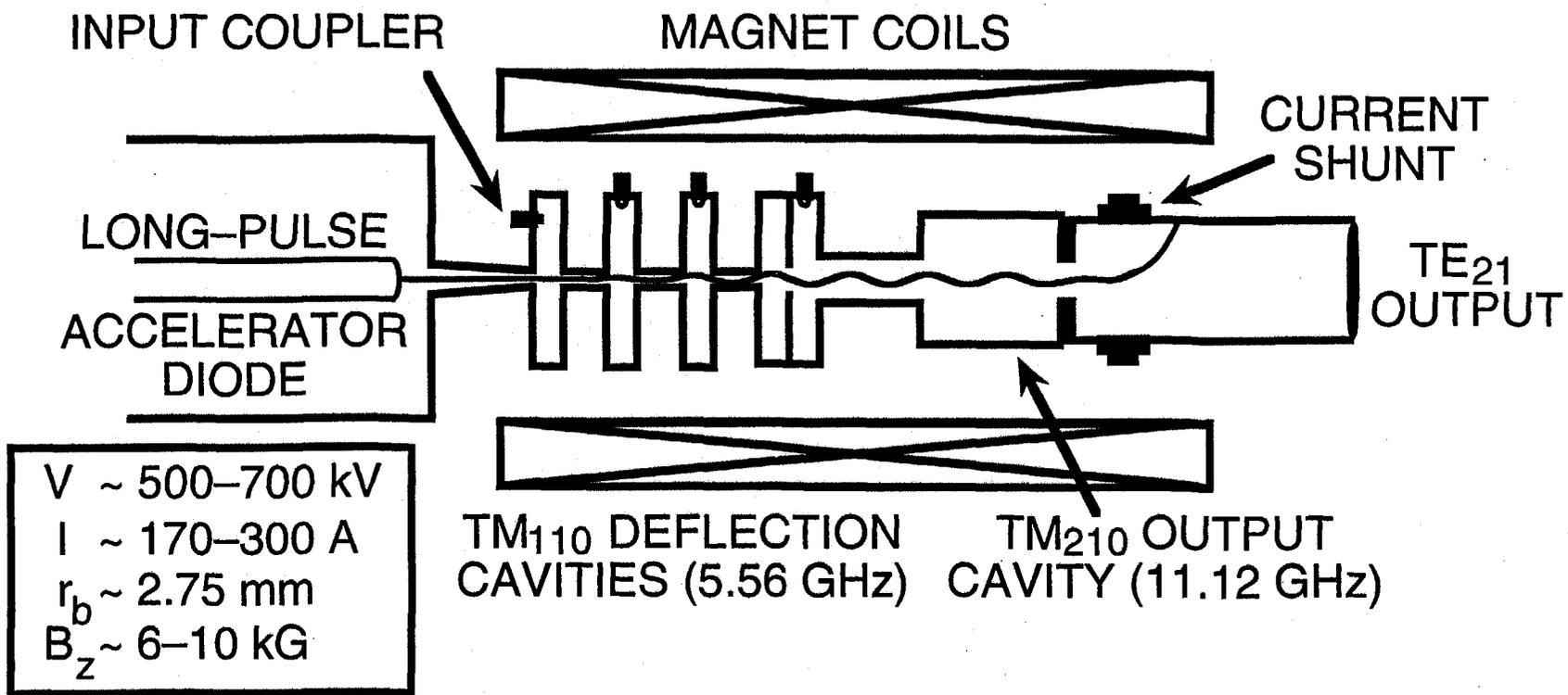
Figure 1. Schematic design of the NRL X-band frequency-doubling magnicon amplifier
