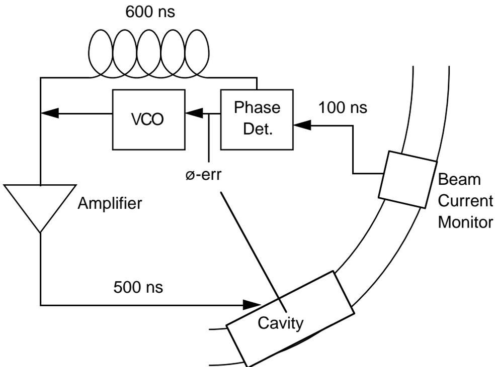
**Figure 1.** Block diagram of the Main Ring beam phase feedback system. Notice that the phase error at the phase detector will match the phase difference between the VCO and the beam at the cavity.
