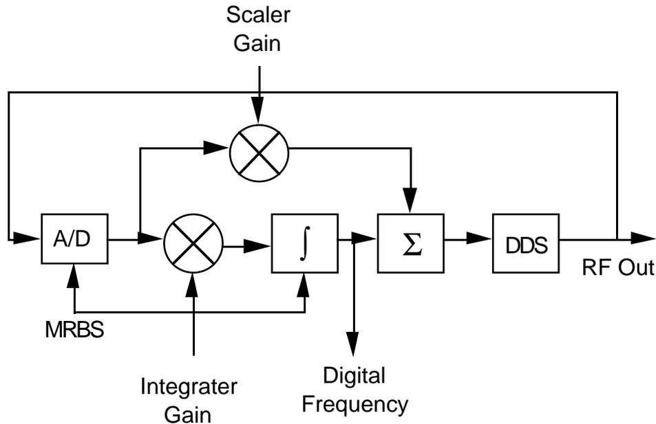
**Figure 4.** RF regeneration circuit. RF phase locks to the MRBS and produces the digital frequency signal necessary to drive the phase shifter.
