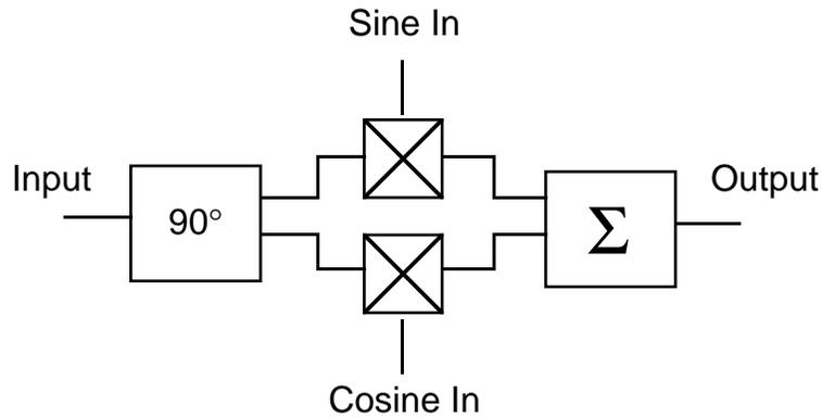
**Figure 2.** I & Q Phase Modulator. The cosine and sine inputs are driven by a voltage which is proportional to the real and imaginary parts of the output signal desired.
