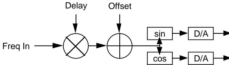
**Figure 3.** I & Q modulator driver circuit. A digital frequency input will produce two analog signals which are proportional to the real and imaginary parts of the phase shift required.
