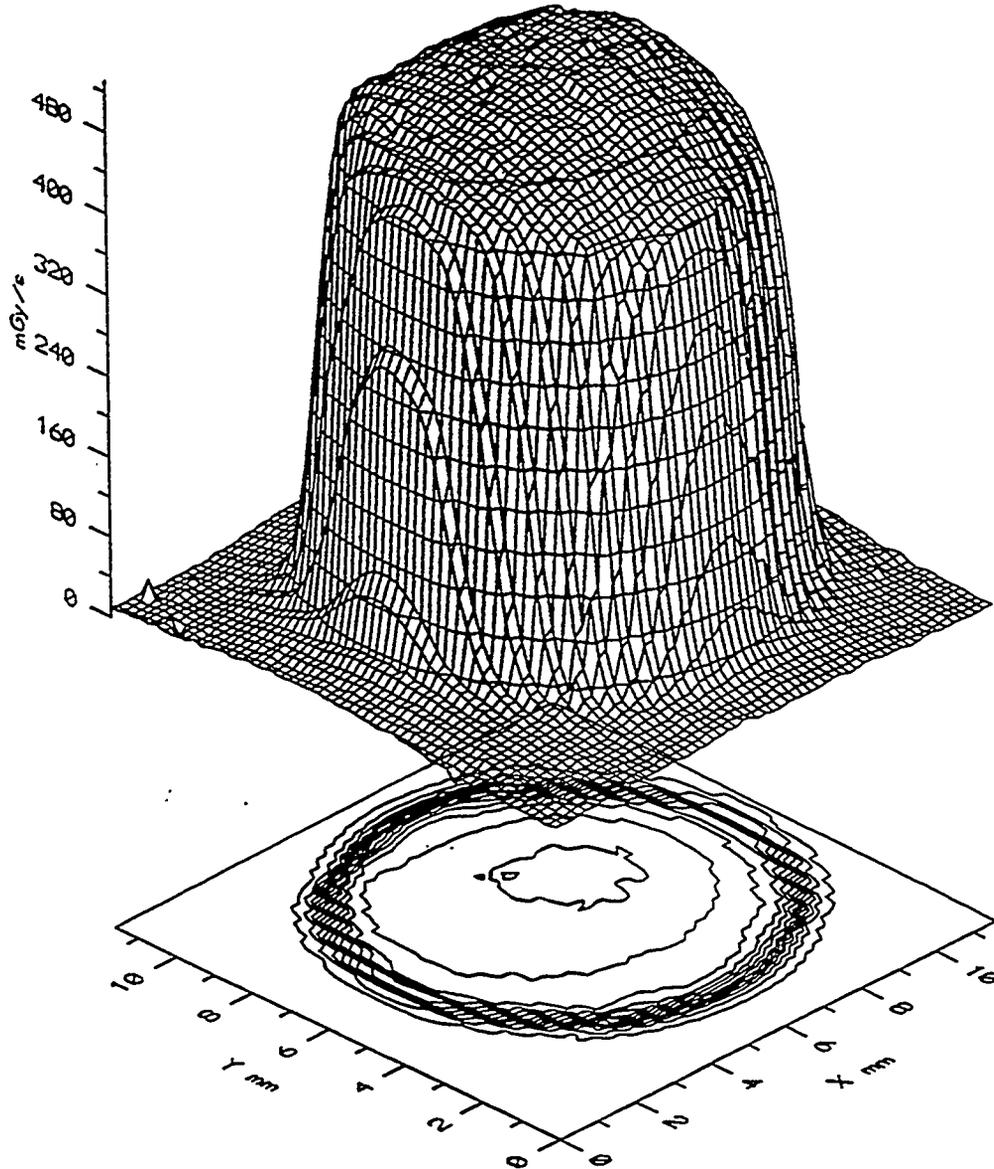
Figure 10 - Isodose Plot and Three-Dimensional Dose Plot for  $^{90}\text{Sr}$ - $^{90}\text{Y}$  Ophthalmic Applicator.
