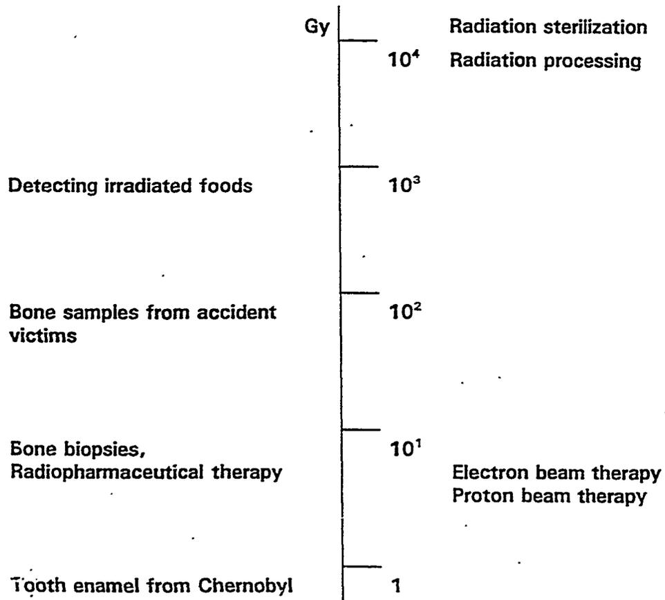
Figure 12 - Electron Spin Resonance Dosimetry (also known as Electron Paramagnetic Resonance Dosimetry), Shown for In Vivo Dosimetry in Bone and for Alanine Crystals.
