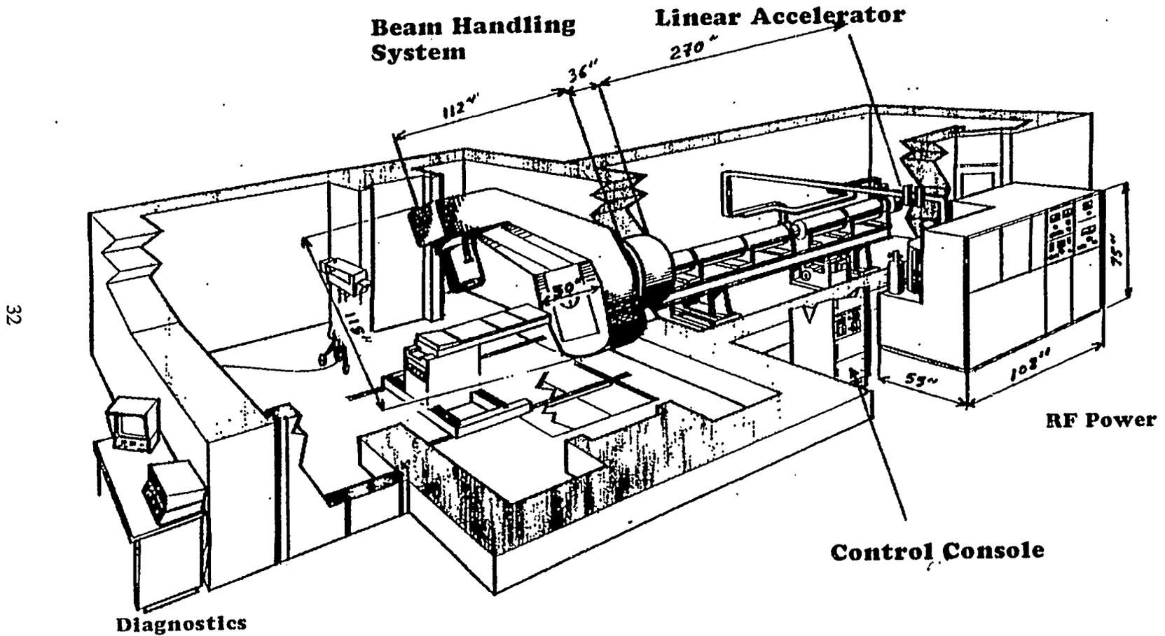
Figure 13 - Layout Diagram for the Sagittaire Linear Accelerator Being Used for the NIST Medical-Industrial Radiation Facility (MIRF).
