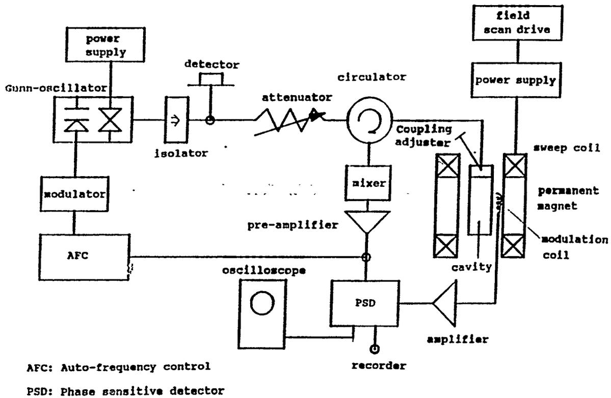
Figure 11 - Block Diagram of a Portable ESR Spectrometer (Kojima et al. 1993).
