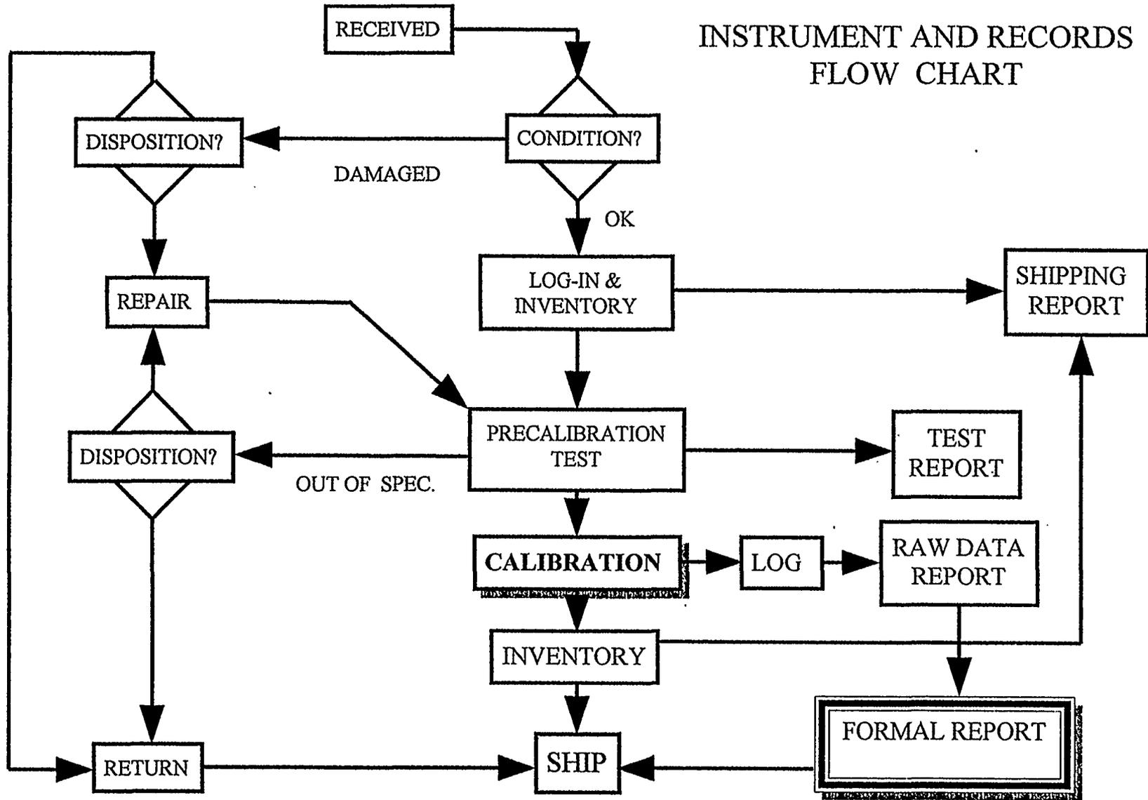
Figure 9 - Instrument and Records Flowchart
