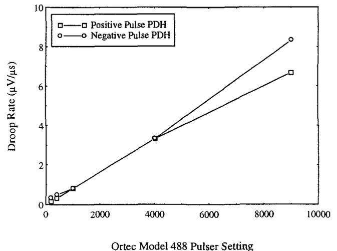
Fig. 7 Droop Rate vs Pulse Amplitude for Negative and Positive PDH Channels
