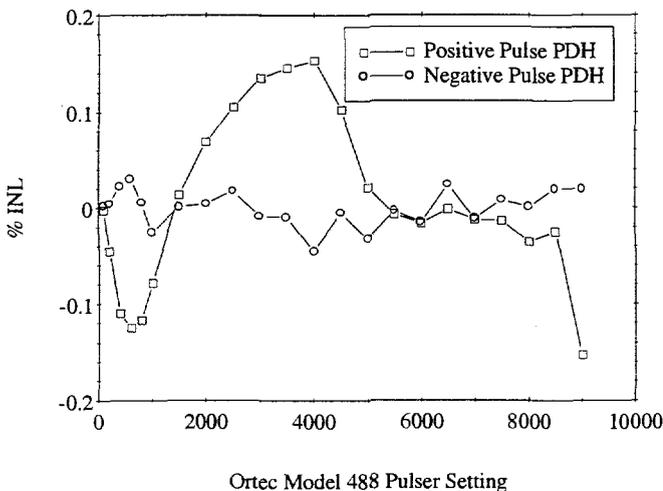
Fig. 5 INL Measurement Results for Positive- and Negative-Pulse PDH Circuits
