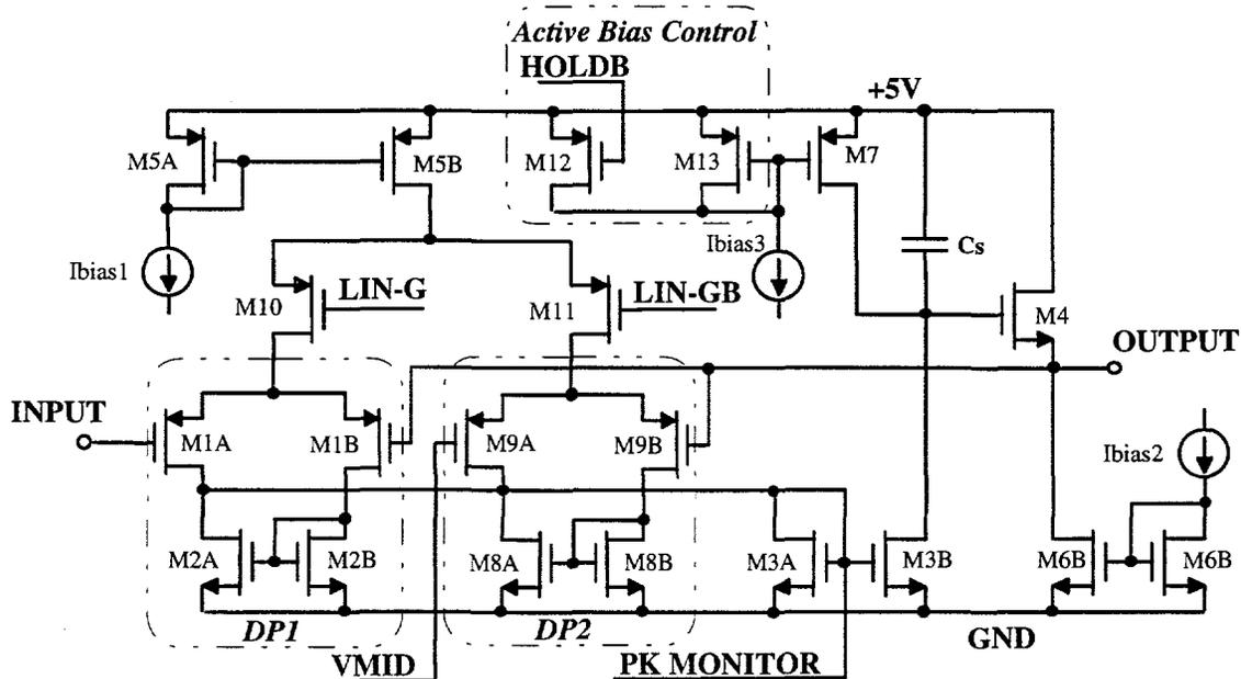
Fig. 3 Improved PDH Circuit Schematic - Negative Pulse Channel
