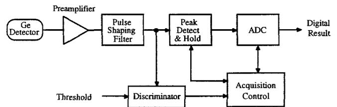
Fig. 2 Nuclear Spectroscopy Pulse Processing and Data Acquisition System Block Diagram
