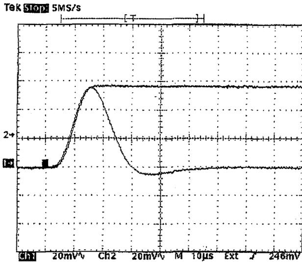
Fig. 4 Sample Input/Output Waveforms for Positive Input PDH Channel
