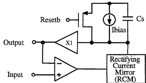
Fig. 1 Peak Detect and Hold Circuit Topology
