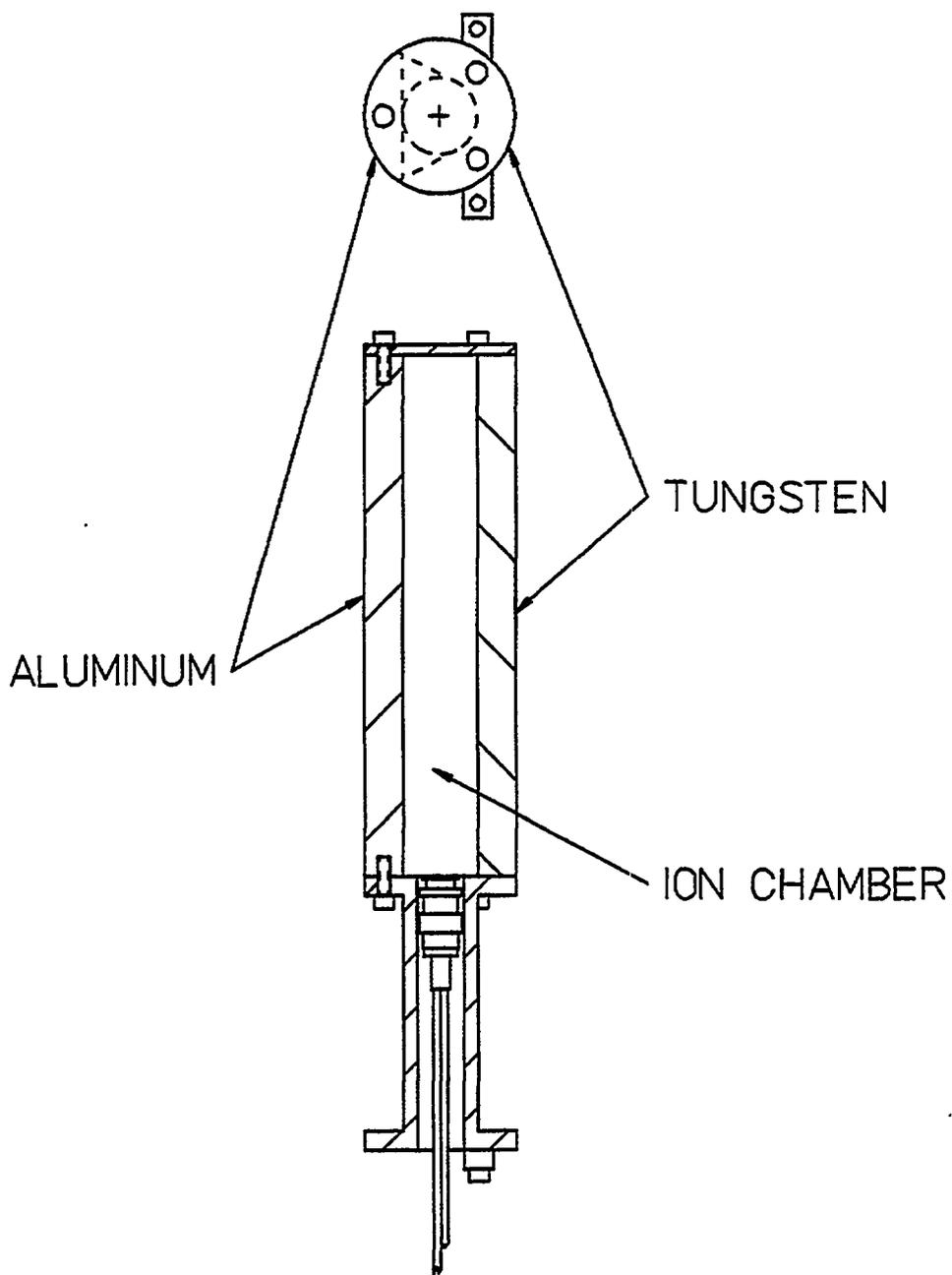
Fig. 6. Schematic of the ion chamber assembly.
