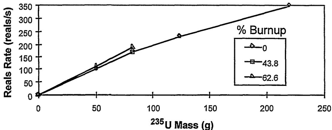
Fig. 16. Example calibration curve for spent fuel.
