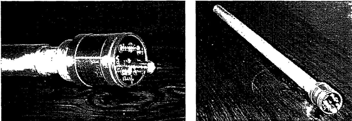
Fig. 5. Photographs of a  $^3\text{He}$  tube with attached preamplifier.
