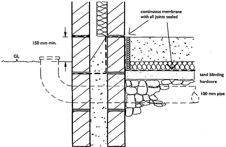
**Figure 4: Hollow Block/Floating Slab**
