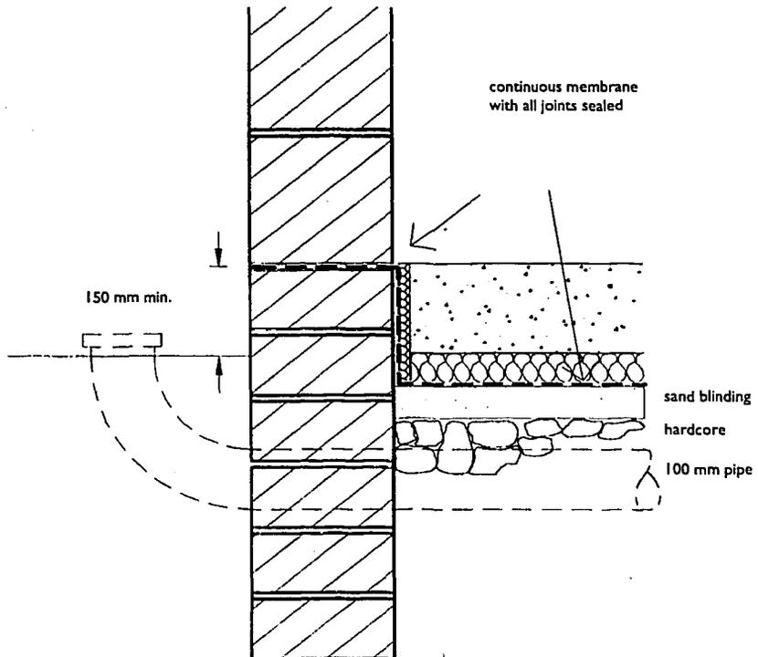
**Figure 5: Suspended Slab**
