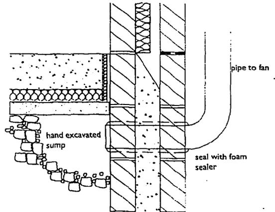
**Figure 14: Centrally Located Sump**
