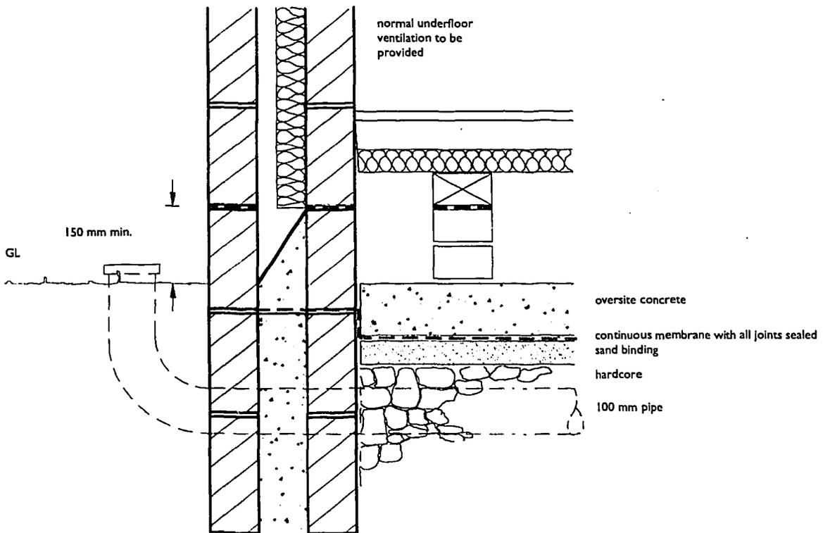
**Figure 7: Membrane at Internal Walls**
