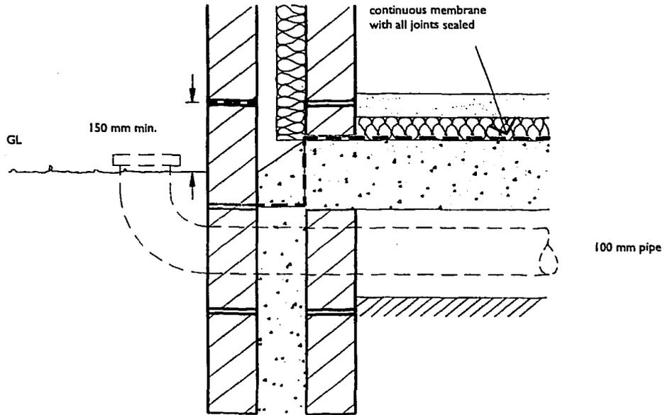
**Figure 6: Suspended Timber Ground Floor Junction with External Wall**
