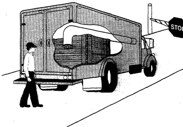
Fig. 4. Conceptual illustration of an LRAD-based vehicle monitor. The air inside the vehicle is recirculated through the ionization detector during a measurement.
