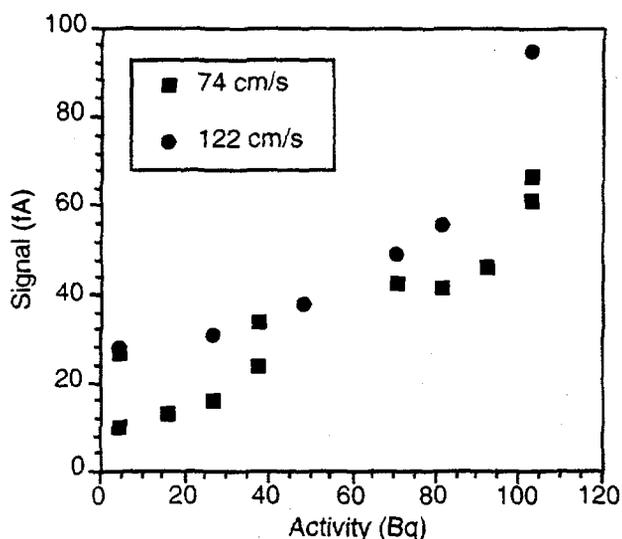
Fig. 5. Efficiency as a function of alpha activity in a measurement through 5 cm of propellant. Note that the efficiency is greater at the higher airspeed.
