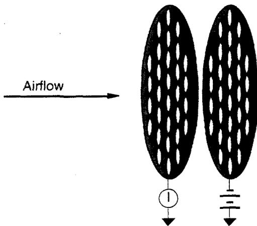
Fig. 1. Illustration of double perpendicular grid ion detector design. The air must pass through the holes in the grid structure.
