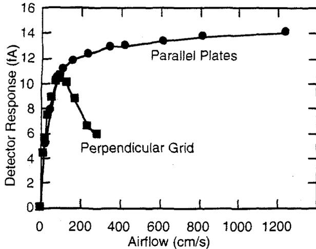
Fig. 3. Response of the perpendicular grid and parallel plate ion detectors as a function of airflow. A small Pu-239 source was located 61 cm. in front of each detector.
