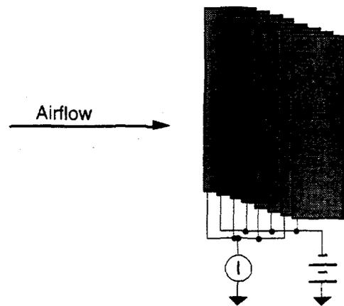
Fig. 2. Parallel plate (high air flow) ion detector. The airflow is much less restricted by this structure than by the grid structure shown in Fig. 1.
