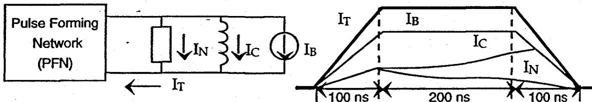
FIGURE 2. Equivalent circuit of an induction cell.
