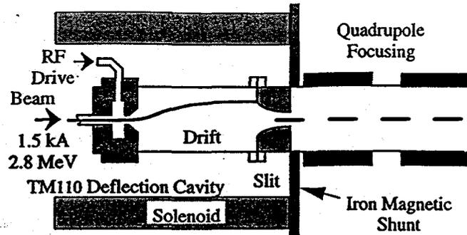
FIGURE 8. Schematic of the RTA beam modulator (chopper).
