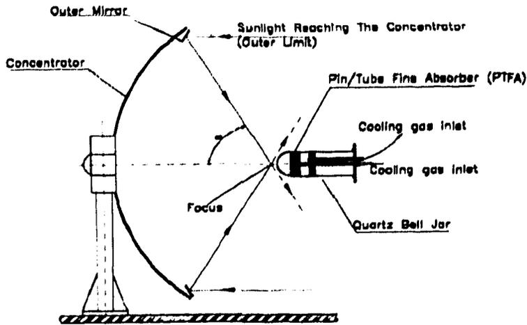
Fig. 4: A Schematic View of the "Solar Furnace" Facility
