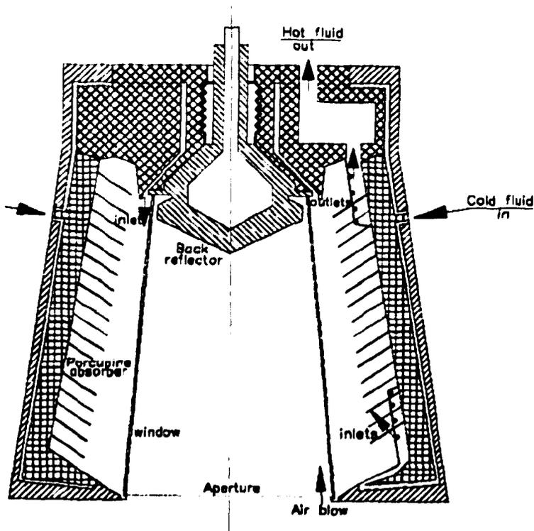
Fig. 16: Schematics of Air Streams within the Receiver
