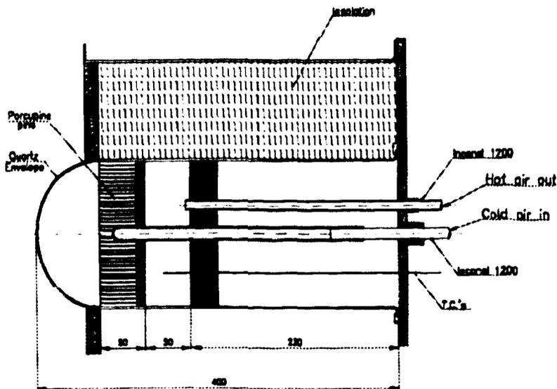
Figure 5a: A Device to Expose Various Absorbers to High Solar Flux
