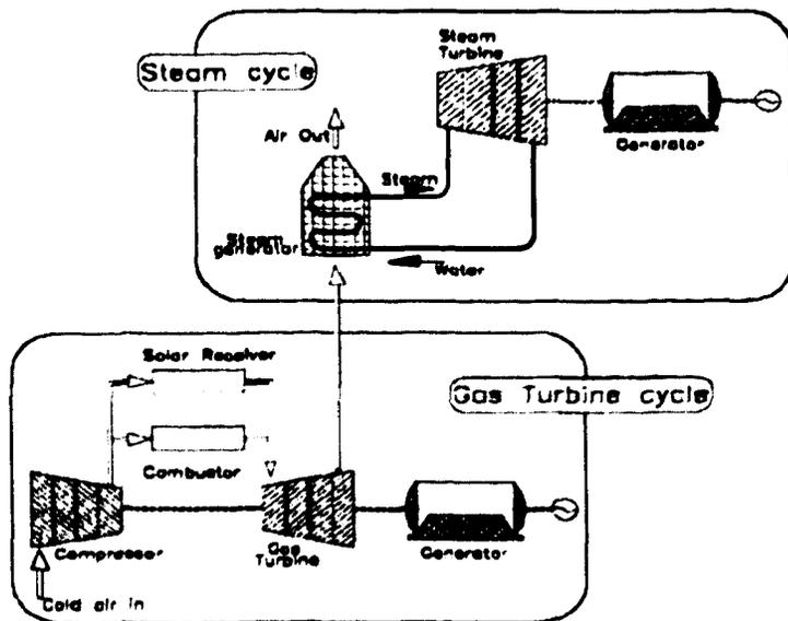
Fig. 1: A Solar-Fossil Combined Cycle Scheme
