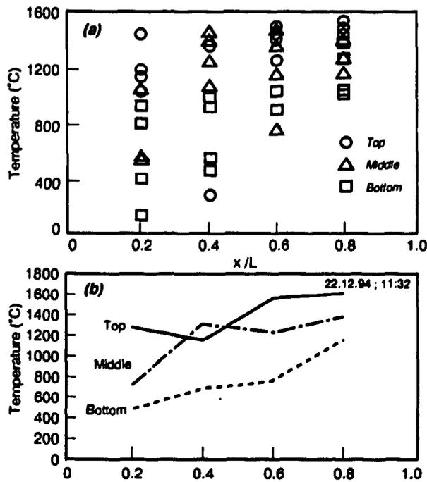
Fig. 19: Examples of Temperature Distribution Over the Absorber in an Actual Test
