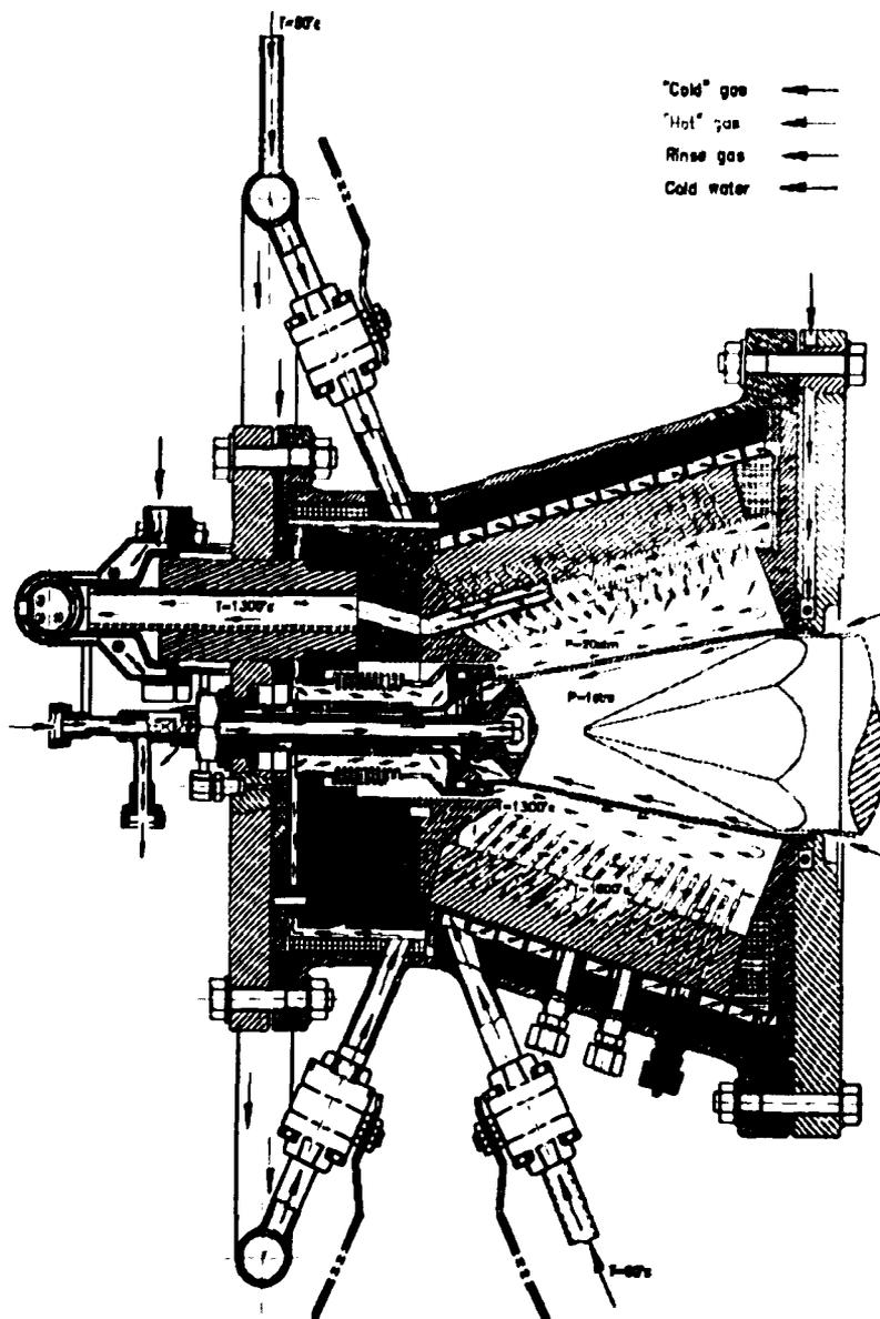
**Fig. 17: Receiver Design with Air Flow Directions and Typical Working Temperatures**
