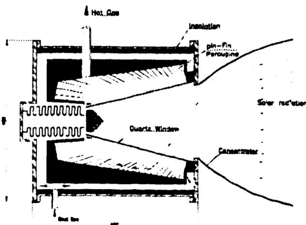
*Fig. 3: A Schematic Layout of the "Porcupine" Receiver.*
