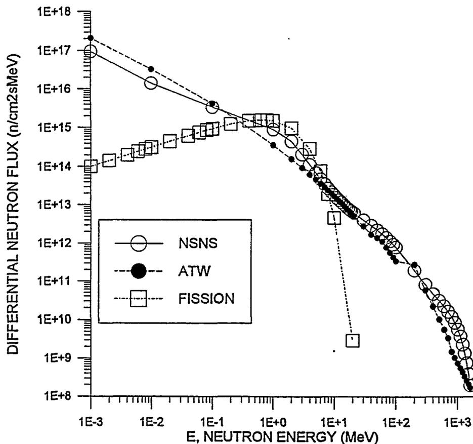
FIG. 1. Neutron spectra that we used for NSNS and ATW, and the prompt fission spectrum for comparison, all normalized to  $\phi(\text{tot}) = 4.2 \times 10^{15}$  n/cm<sup>2</sup>s.
