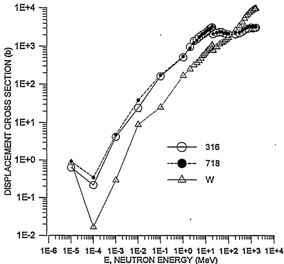
FIG. 2. Displacement cross section vs neutron energy for W, 316 stainless steel, and Inconel 718 as calculated by SPECTER ( $E < 20 \text{ MeV}$ ) and LAHET ( $E > 20 \text{ MeV}$ ).
