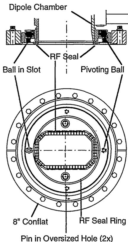
Figure 2. Flex Flange Assembly with Integral RF Seal
