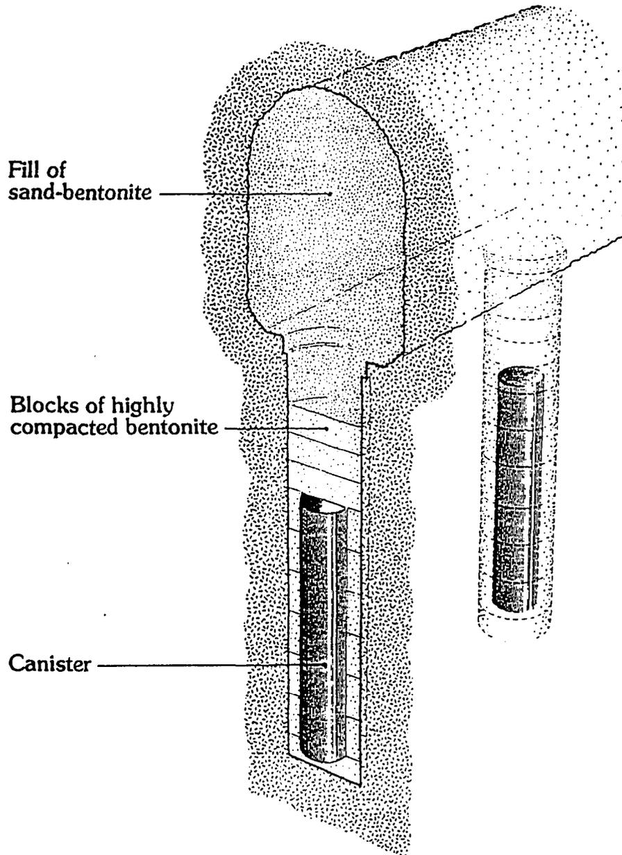
Figure 3. ACP-canister in deposition tunnel
