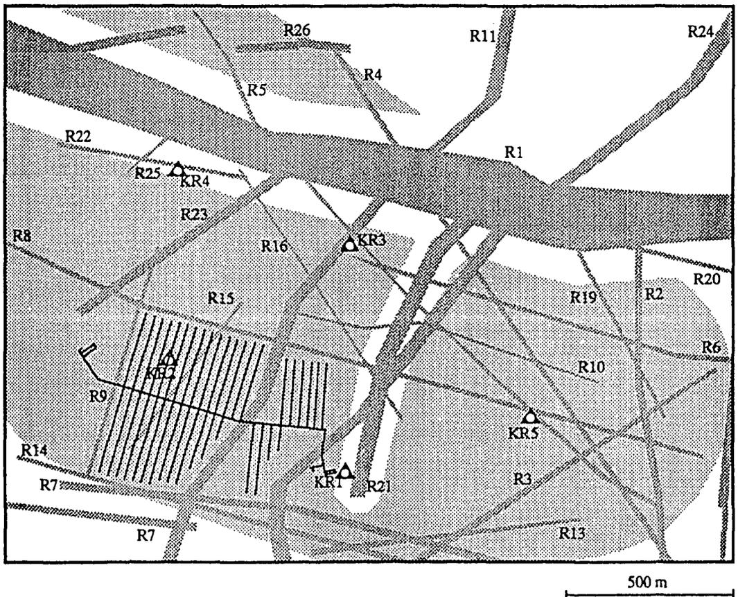
Figure 5. Example showing how the repository can be adjusted to local fracture zones (Veitsivaara).
