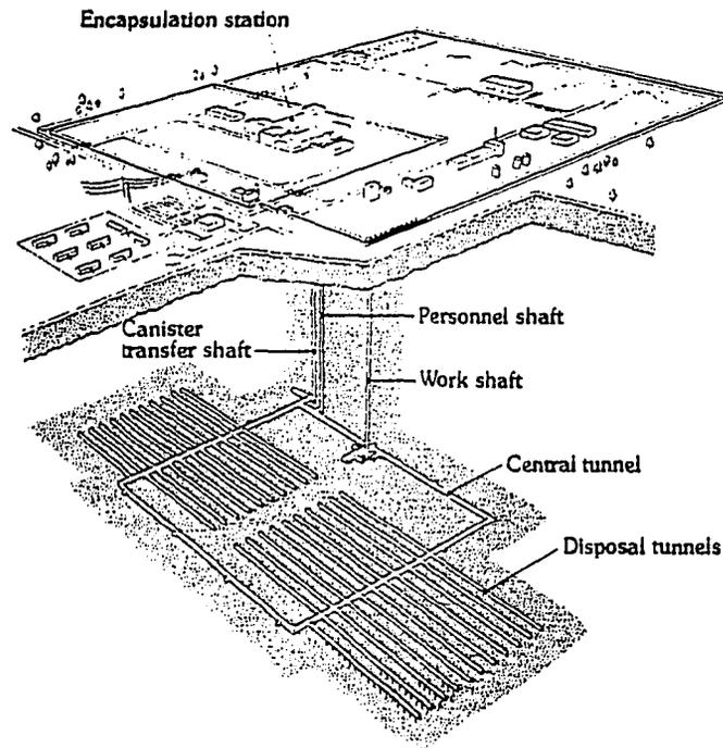
Figure 2. The planned final disposal facility for TVO's spent fuel
