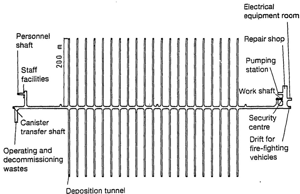
Figure 4. Alternative layout for the final repository.
