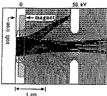
Fig. 3 Planar calculation showing the effect of the extracted electrons due to a pair of permanent magnets located inside the first electrode.
