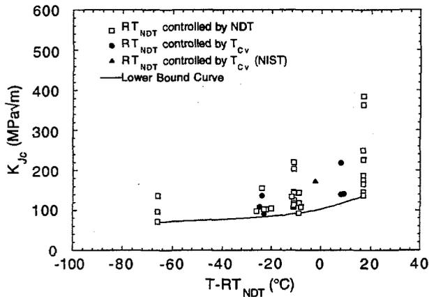
Fig. 7. The parameter controlling  $RT_{NDT}$  has no significant effect on the distribution of  $K_{Jc}$  vs  $T-RT_{NDT}$  data points from the deep-crack SENB A533B specimens. A single curve adequately defines the lower bound for the combined data set
