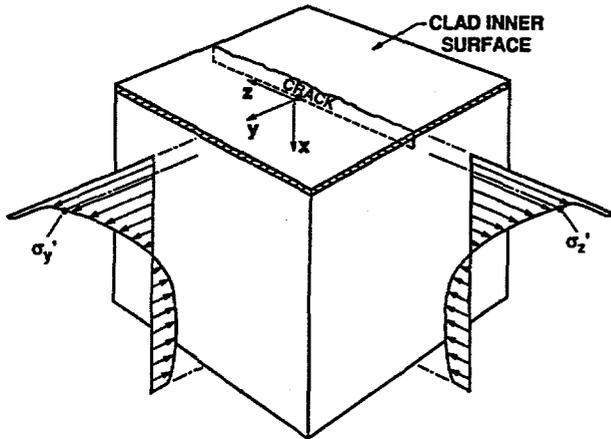
Fig. 1. PTS loading biaxial stresses in a reactor vessel wall with one of the principal stresses aligned parallel with the tip of a constant-depth shallow surface flaw
