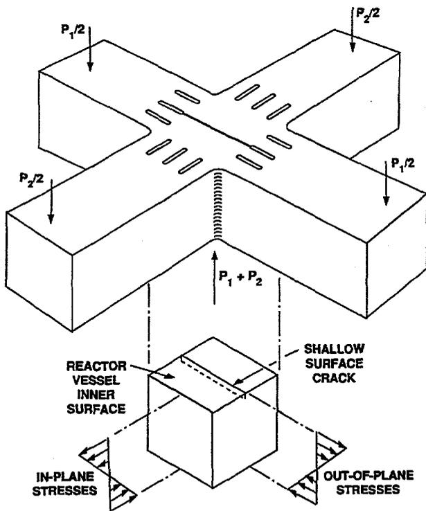
Fig. 10. Conceptual features of the cruciform shallow-flaw biaxial fracture toughness test specimen
