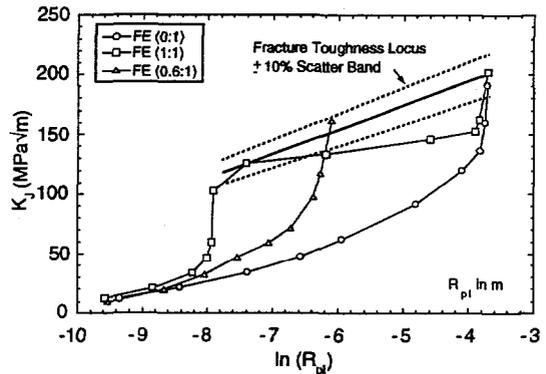
Fig. 22. Equivalent  $K_J$ ,  $K_{Jc}$  vs  $\ln(R_{pl})$  relationships for cruciform testing program
