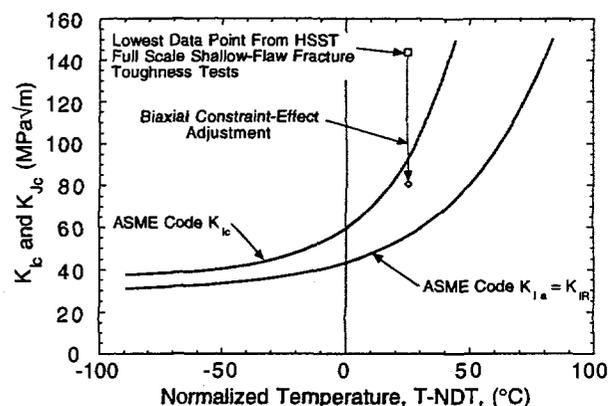
Fig. 17. The lowest data point from the full-scale uniaxial shallow-flaw fracture-toughness tests on weld material is located below the ASME  $K_{Ic}$  curve but above the  $K_{IR}$  curve when adjusted for the possible effects of biaxial loading
