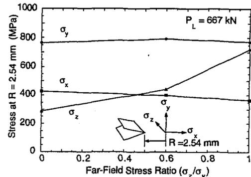
Fig. 3. Far-field stress biaxiality has little effect on the in-plane stresses near the crack tip
