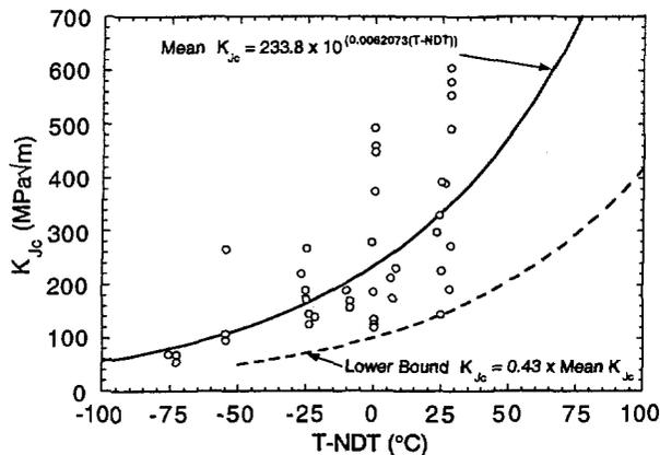
Fig. 12. Mean and lower bound  $K_{Jc}$  curves derived from the uniaxial shallow-flow fracture toughness data and used in the RPV PTS analysis
