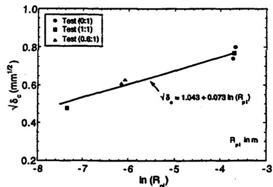
Fig. 18. Analyses of cruciform data imply  $\sqrt{\delta_c}$  is linearly related to  $\ln(R_{pl})$
