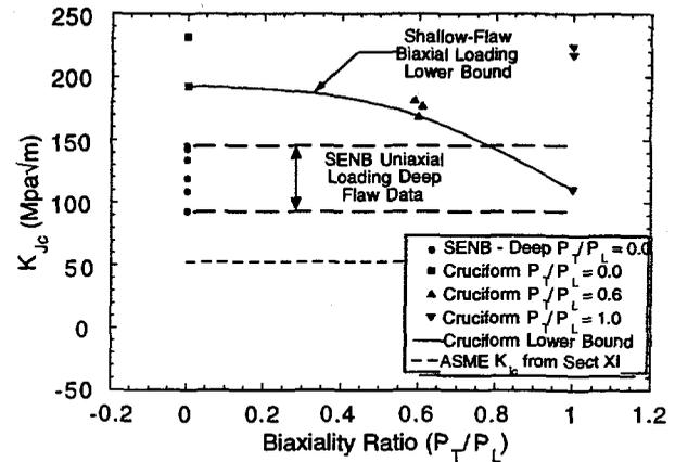
Fig. 11. Data from a single heat of A533B steel tested at  $T\text{-NDT} = -10^\circ\text{C}$  indicate that biaxial loading reduces the lower-bound transition-range shallow-flaw fracture toughness
