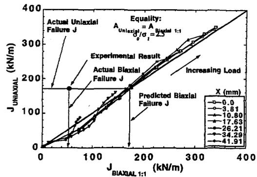
Fig. 4. Validation check on the Dodds-Anderson constraint adjustment for data from biaxial ( $P_T/P_L = 1.0$ ) and uniaxial ( $P_T/P_L = 0.0$ ) tests
