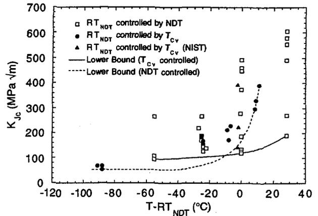
Fig. 8. Shallow-flaw fracture toughness data for A533B plate and weld material fall into two distinct groups when plotted as a function of the normalizing parameter  $T-RT_{NDT}$ . The groups are characterized by the parameter controlling  $RT_{NDT}$  (NDT or  $T_{Cv}$ )
