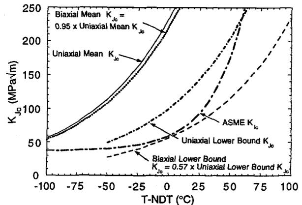
Fig. 13. Mean and lower-bound  $K_{Jc}$  curves adjusted to reflect the effect of  $P_T/P_L - 1.0$  loading biaxiality on shallow-flow fracture toughness
