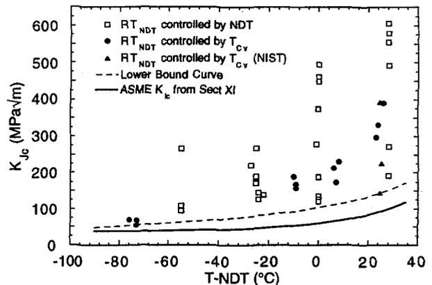
Fig. 9. Shallow-flaw fracture toughness data for A533B plate and weld material from a single homogeneous group when plotted as a function of the normalizing parameter  $T-NDT$ . The lower bound curve of this data set is similar to that of the deep flaw data set, but the shallow-flaw data set show an increase in both mean toughness and data scatter
