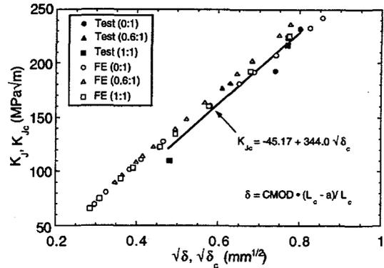
Fig. 21. The linear relationship between  $K_J$  and  $\sqrt{\delta}$  is maintained for all biaxial loading ratios
