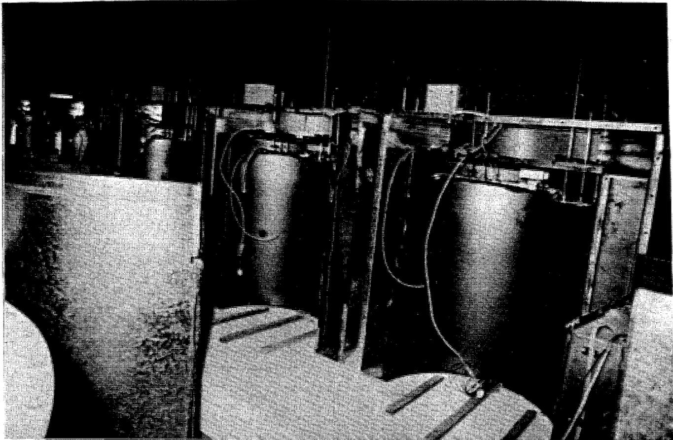
Figure 2. Internal View of Gas Generation Test Assemblies.
