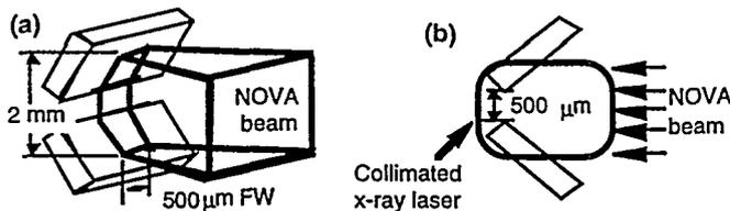
Fig. 1 The colliding plasma experimental setup. (a) 3-D view of Nova beam illuminating the 2 Au slabs. (b) side view showing the window of collimated x-ray laser beam which defines the view of the gated detector.
