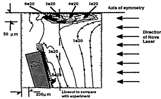
Fig. 3 A snapshot of a LASNEX-calculated 2-D  $n_e$  profile at a time of 150 ps after optical laser pulse. This time corresponds to the peak of the x-ray laser pulse that served as the gate for our imaging detector used for the experiment.
