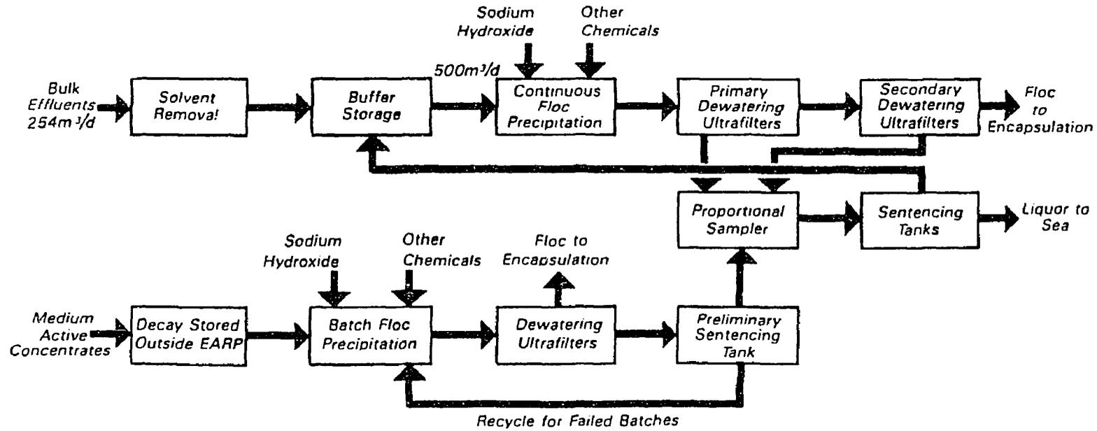
Figure 6 EARP - Simplified Process Flow Diagram
