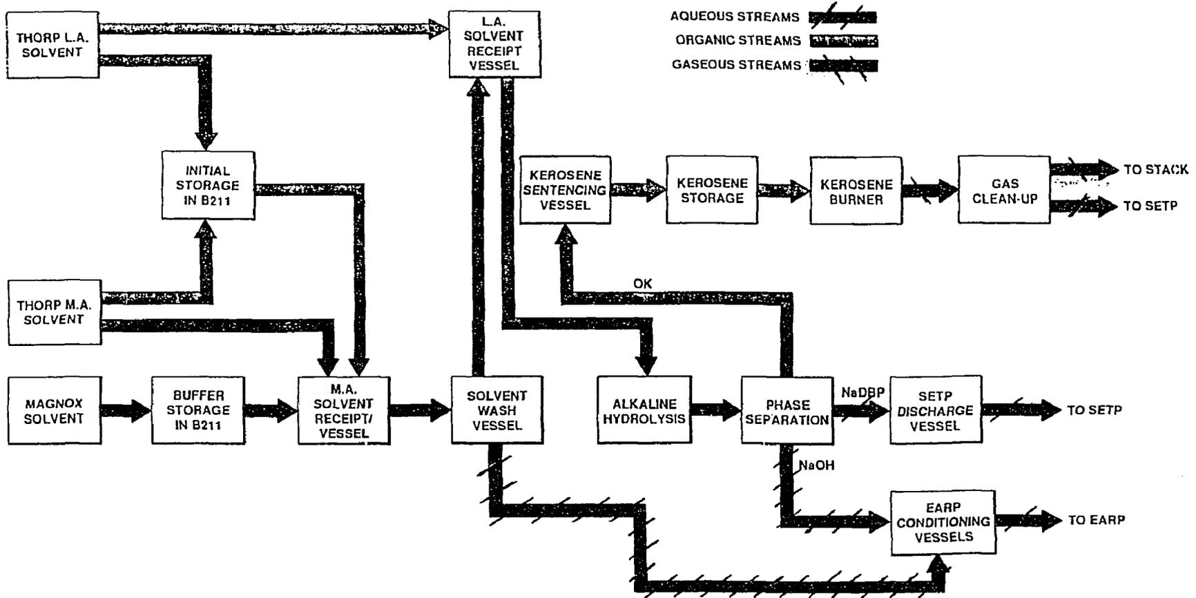
Figure 7 STP Block Flow Diagram
