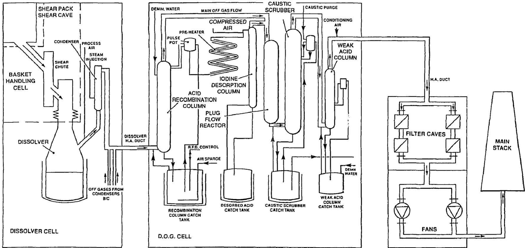
Figure 3 Dissolver off gas (DOG) extract system
