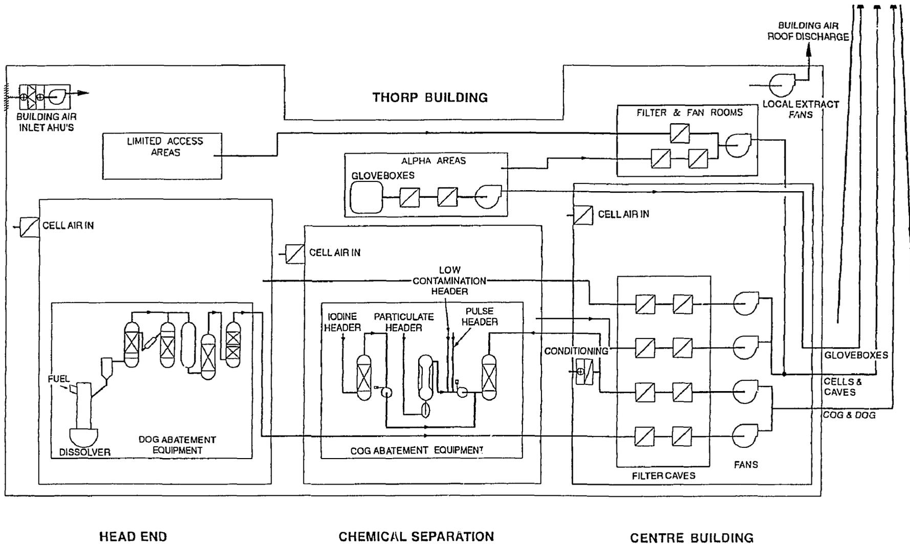
Figure 2 Schematic of THORP active ventilation systems
