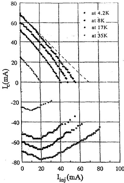
Fig.3 YBCO thin film current  $I_c$  as a function of injection current  $I_{inj}$  at different temperatures.
