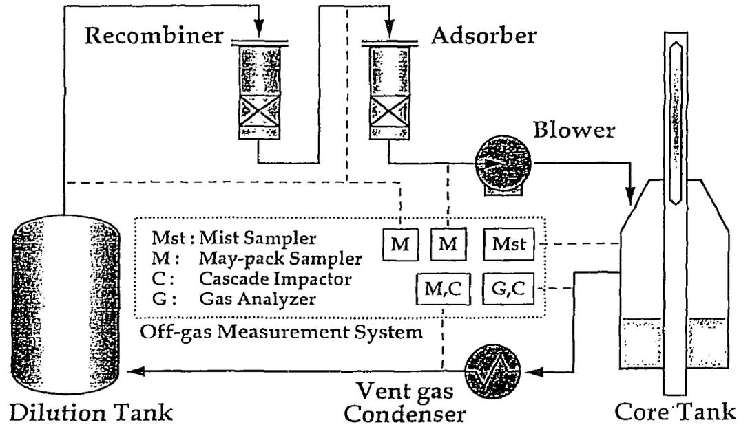
Fig. 6 Off-gas Ventilation System
