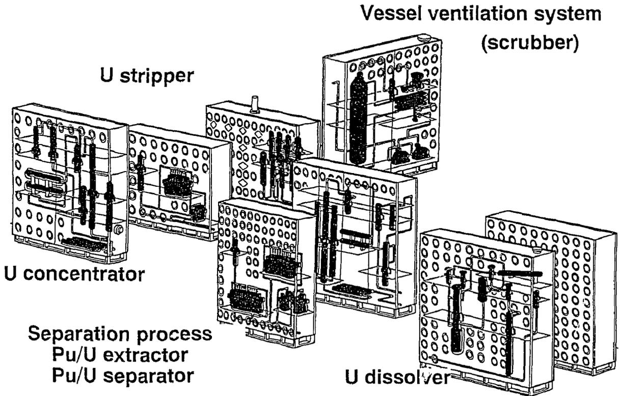
Fig. 7 Layout of Fuel Treatment System
