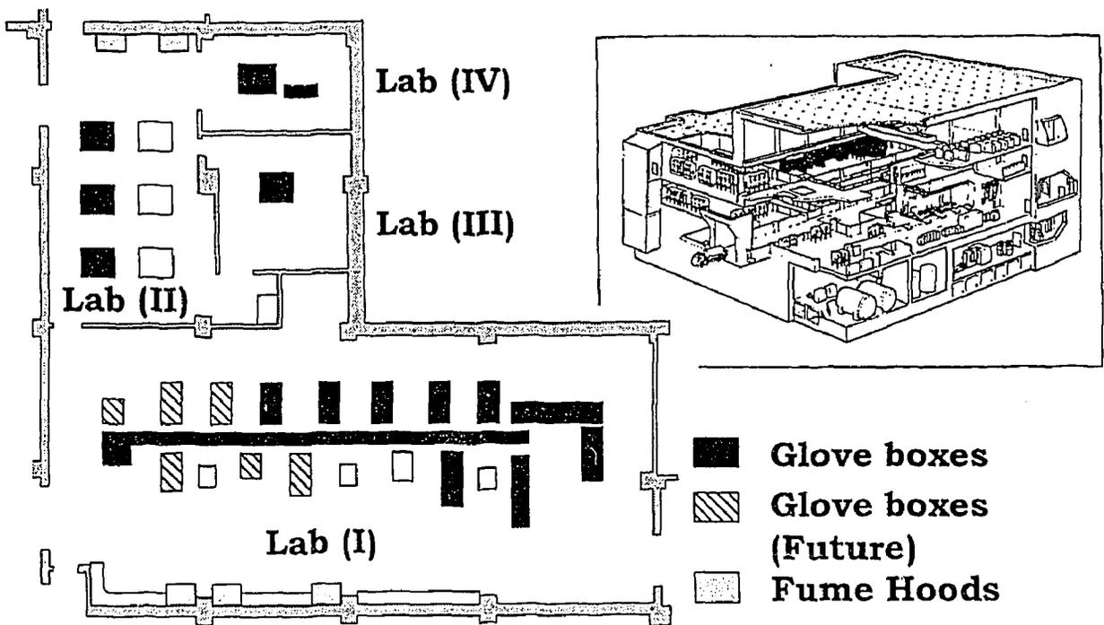
Fig. 8 Layout of Analytical Laboratories and Instruments
