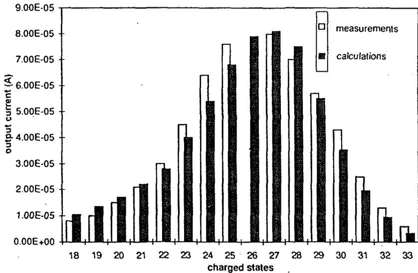
**Figure 5.** Calculated charge state distribution of lead ion in the afterglow mode of ECR ion source in comparison with experimental data
