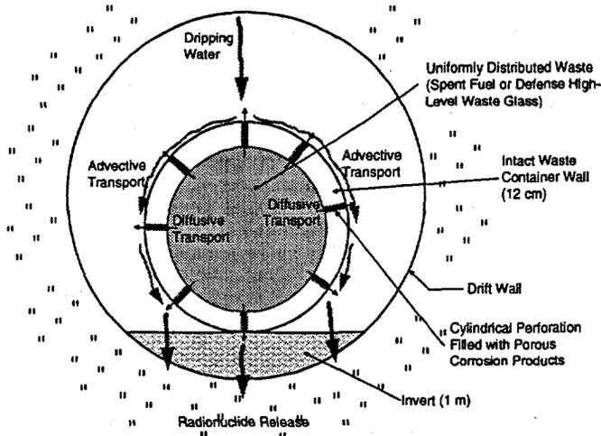
Figure 2 Schematic of the EBS advective release model II (Drip-on-Waste-Package Model) in which the dripping water is diverted around the waste package, and radionuclides are transported by diffusion through the perforations in the waste container, then are released by advection.
