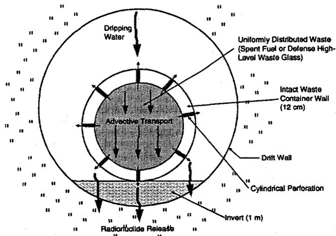
Figure 1 Schematic of the EBS advective release model I (Drip-on-Waste-Form Model) in which the dripping water directly contacts the waste form, and radionuclides are released by advection through the waste package.
