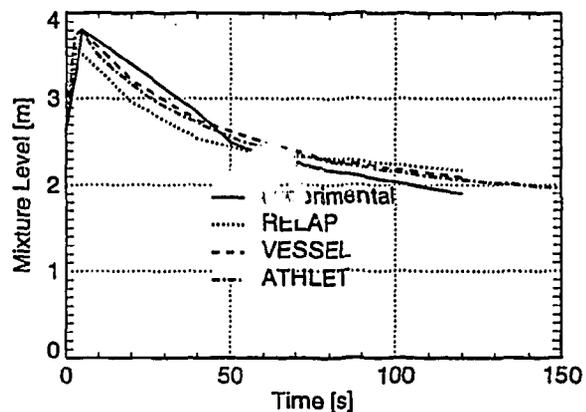
Fig. 4 Time dependent mixture level in the vessel
