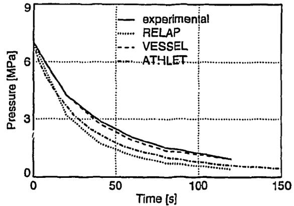
Fig. 3 Time dependent pressure in the vessel
