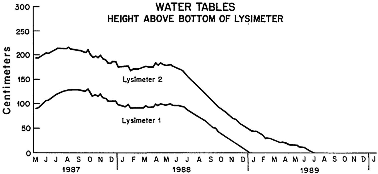
Fig. 8. Water table vs. time in bioengineered lysimeters. Decline of water-table levels with time shows bioengineered covers effectively prevented water percolation. Elimination of water table shows that this procedure could be used for remedial action ("drying out") of existing water-logged burial sites. Compare with Fig. 7.
