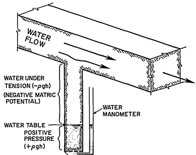
Fig. 20. Schematic of laboratory apparatus for measurement of water tension using different materials and varying flow rates.
