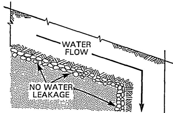
Fig. 18. Substitution of rock layer for holes shown in Fig. 17. Voids between rocks act exactly like holes shown in Fig. 17. They form a capillary discontinuity, preventing leakage downward under the influence of gravity.
