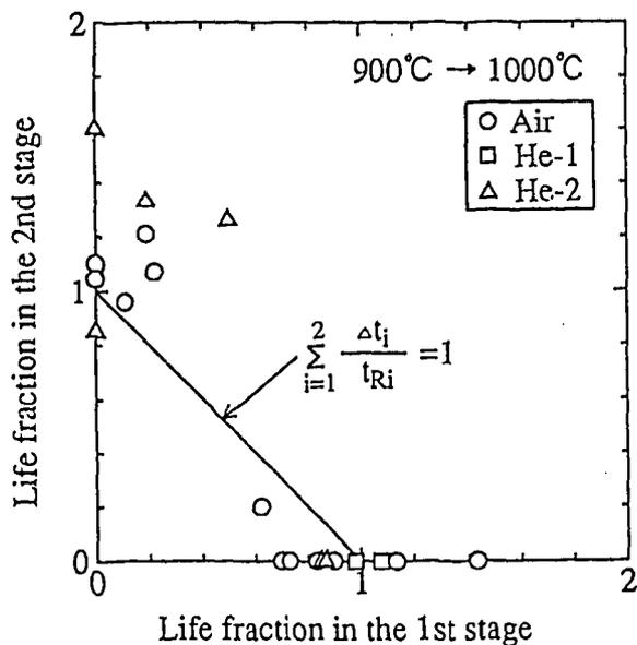
Fig. 5 Result of application of the life fraction rule to the test results under the conditions from 900 to 1000°C for Hastelloy XR with 60 mass ppm boron.
