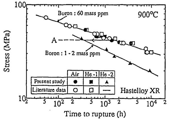
Fig. 10 Relation between applied stress and time to rupture obtained with constant load and temperature creep rupture tests for Hastelloy XR whose boron content levels are different. The figure includes the data obtained in another work [7] for the same heat material.
