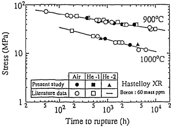
Fig. 3 Relation between applied stress and time to rupture obtained with constant load and temperature creep rupture tests for Hastelloy XR with 60 mass ppm boron. The figure includes both of the data obtained in the present study and in another work [7] for the same heat material.
