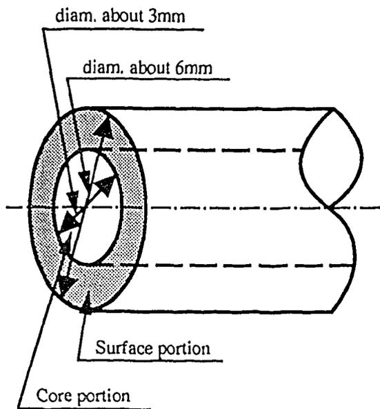
Fig. 7 Schematic illustration of the sampling method of specimens for boron analyses.
