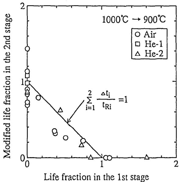
Fig. 12 Result of application of the modified life fraction rule to the test results under the conditions from 1000 to 900°C for Hastelloy XR with 60 mass ppm boron.
