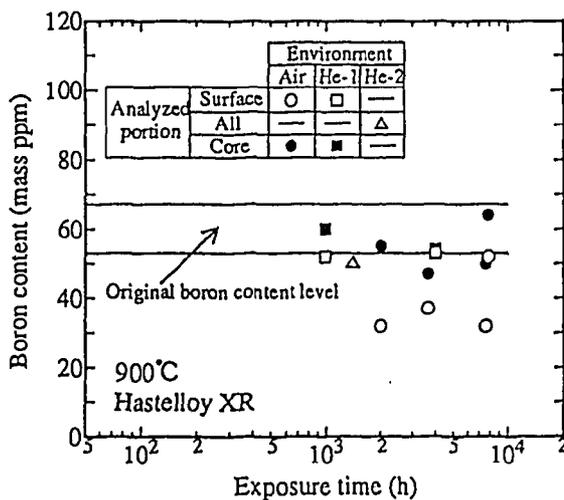
Fig. 8 Results of boron analyses as a function of the exposure time to the high-temperature environments at 900°C. The figure does not include the results under varying load and temperature conditions.
