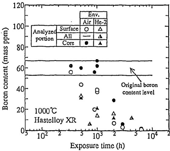
Fig. 9 Results of boron analyses as a function of the exposure time to the high-temperature environments at 1000°C. The figure does not include the results under varying load and temperature conditions.
