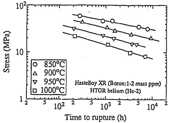
Fig. 2 Relation between applied stress and time to rupture obtained with constant load and temperature creep rupture tests for Hastelloy XR with 1 to 2 mass ppm boron.
