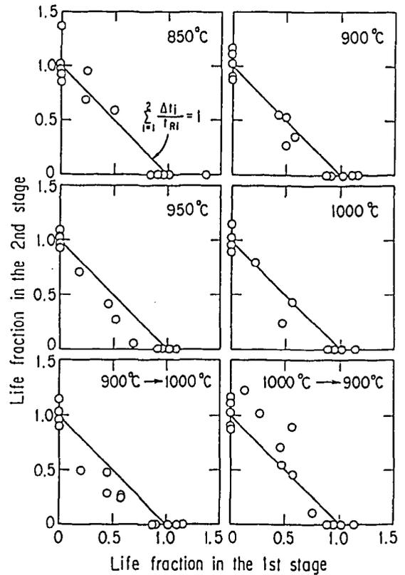
Fig. 4 Result of application of the life fraction rule to the varying stress and/or temperature test results for Hastelloy XR with 1 to 2 mass ppm boron.
