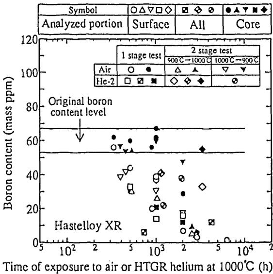
Fig. 11 Results of boron analyses as a function of the exposure time to high-temperature environments at 1000°C. The figure includes the results under varying load and temperature conditions.
