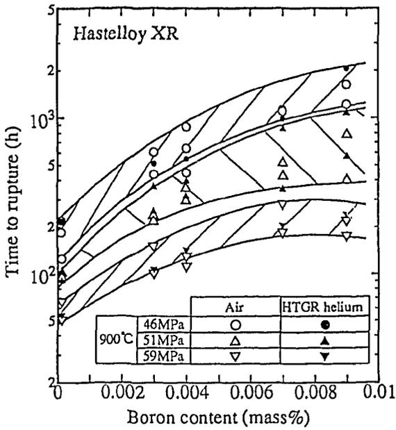
Fig. 1 Effect of the boron content level on the creep rupture life of Hastelloy XR [4].
