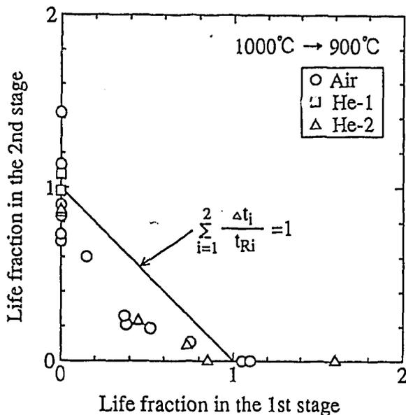
Fig. 6 Result of application of the life fraction rule to the test results under the conditions from 1000 to 900°C for Hastelloy XR with 60 mass ppm boron.
