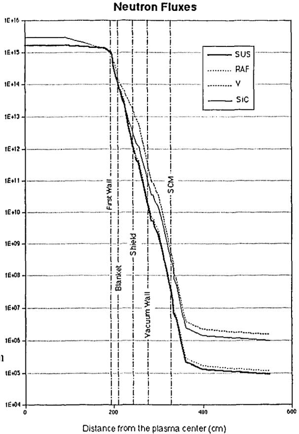
Fig. 5 Neutron flux of 14 MeV as a function of the distance from the plasma center.
