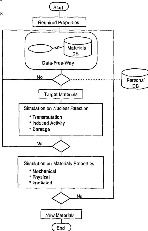
Fig. 1 Flow diagram on the concept of the ata system for nuclear material design and selection.
