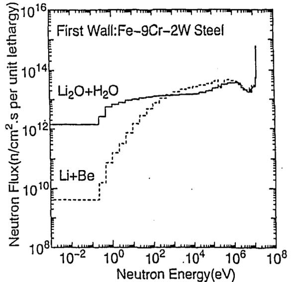
Fig.8 Neutron spectra at the first wall of 9Cr-2W/Li<sub>2</sub>O H<sub>2</sub>O and 9Cr-2W/Li/Be blanket/shield systems.
