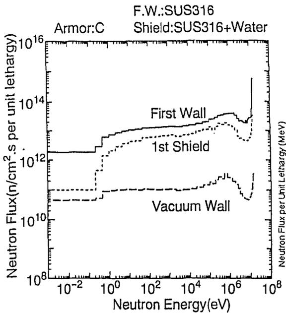
Fig. 4 Neutron spectra at first wall, shield and vacuum position under 1 MW/m<sup>2</sup> wall loading.
