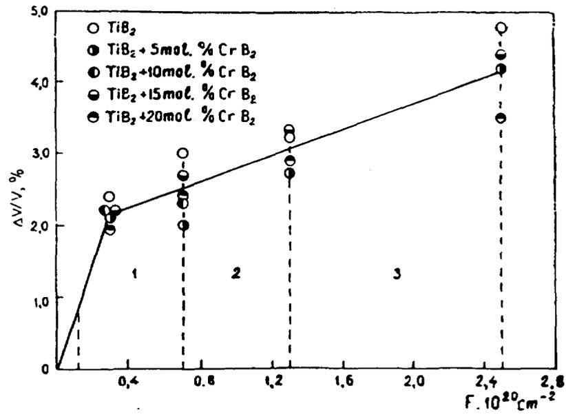
Fig.1. The change of macrovolume  $\Delta V/V$  and damage character of microstructure for  $\text{TiB}_2$  and its alloys with  $\text{CrB}_2$  as function of thermal neutron fluence at the temperature of  $\sim 100^\circ\text{C}$ .
