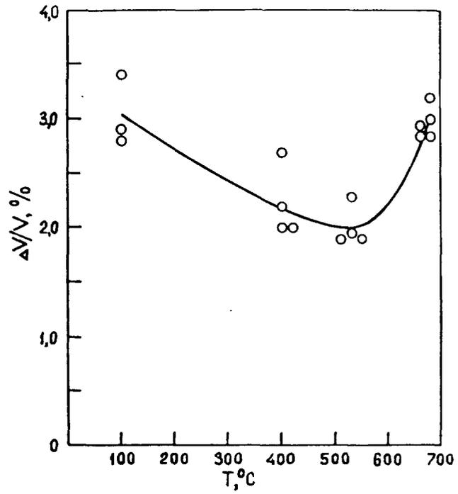
Fig.3 - Dependence of  $\text{TiB}_2$  macrovolume  $\Delta V/V$  upon the irradiation temperature for thermal neutron fluence of  $7,0 \times 10^{19} \text{ cm}^{-2}$ .
