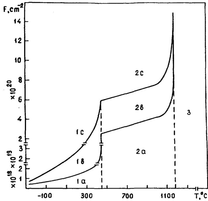
Fig.4 - General scheme of radiation damage and destruction of titanium diboride under neutron irradiation.
