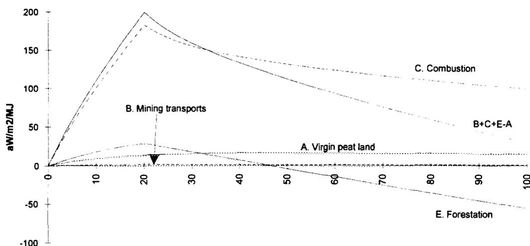
Figure 9. Calculated radiative forcing for the case *peat modified* (Bergslagen): the production and combustion of 1 MJ peat assuming that all drained areas are forested. The contribution from each activity is shown. Values in  $\text{aW/m}^2/\text{MJ}$ .
