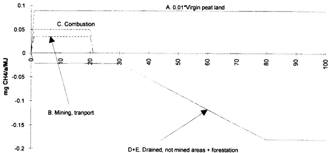
Figure 4. CH<sub>4</sub>-emissions from the production and combustion of 1 MJ peat according to the case *Peat today*, in the region *Bergslagen* [g CH<sub>4</sub>/MJ]. The post *A. Virgin peat land* has been scaled down by a factor 100 in order to make the other posts visible.
