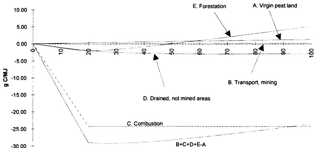
Figure 6. Accumulated CO<sub>2</sub>-emissions from the production and combustion of 1 MJ peat according to the case *Peat today*, in the region *Bergslagen* [g C/MJ].
