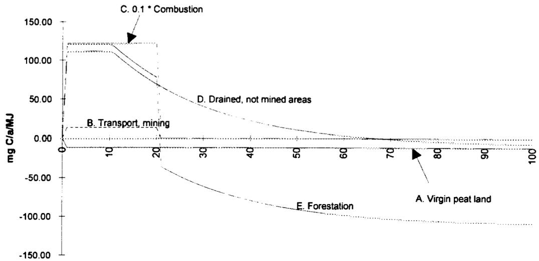
Figure 3. CO<sub>2</sub>-emissions from the production and combustion of 1 MJ peat according to the case *Peat today*, in the region *Bergslagen* [g CO<sub>2</sub>-C/MJ]. The post *C. Combustion* has been scaled down by a factor 10 in order to make the other posts visible.
