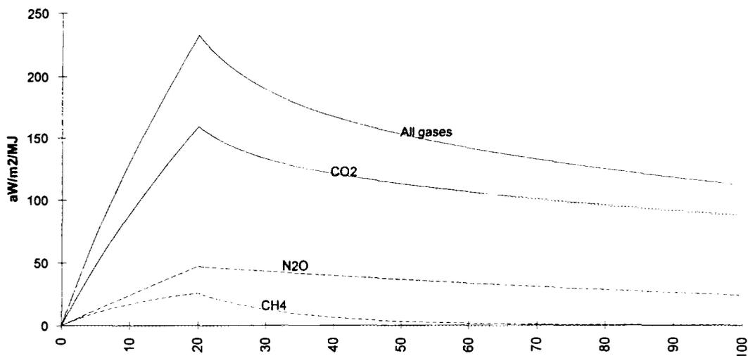
Figure 10. Calculated radiative forcing for the case *coal today*: the mining and combustion of 1 MJ coal as it is done today. The contribution from each greenhouse gas is shown. Values in aW/m<sup>2</sup>/MJ coal.
