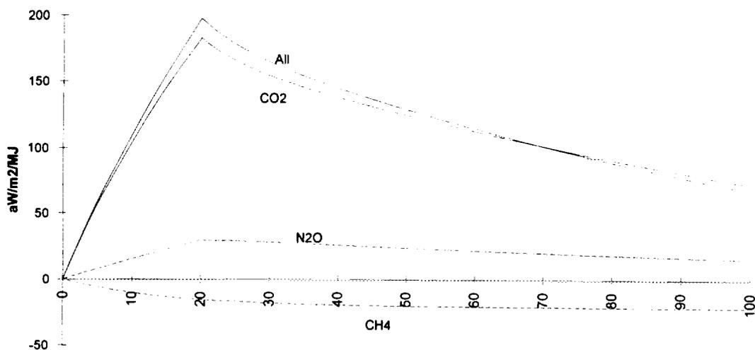
Figure 7. Calculated radiative forcing for the case *peat today* (*Bergslagen*): the production and combustion of 1 MJ peat as it is done today. The contribution from each gas is shown. Values in  $\text{aW/m}^2/\text{MJ}$ .
