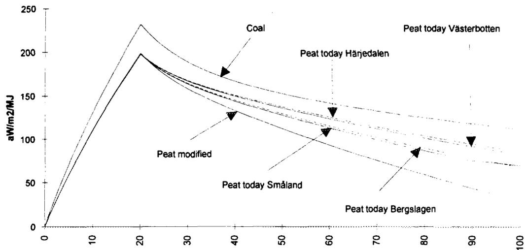
Figure 11. Radiative forcing for the different cases. Values in  $\text{aW/m}^2/\text{MJ}$ .
