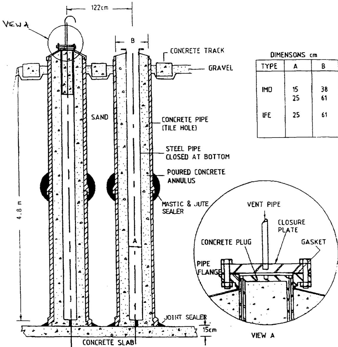
Figure 3. Typical Fuel Storage Tile Holes
