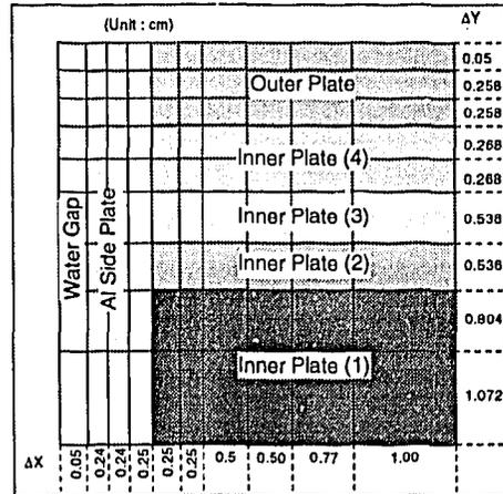
Fig.-5 Element Cell Calculation Model
