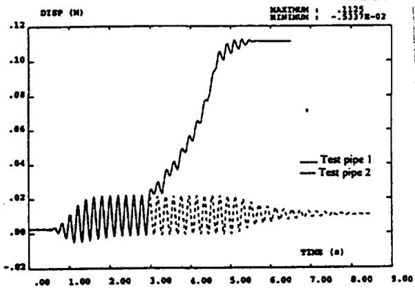
FIG. 6 : TESTS DISPLACEMENT CRACKED PIPE 1 AND PIPE 2
