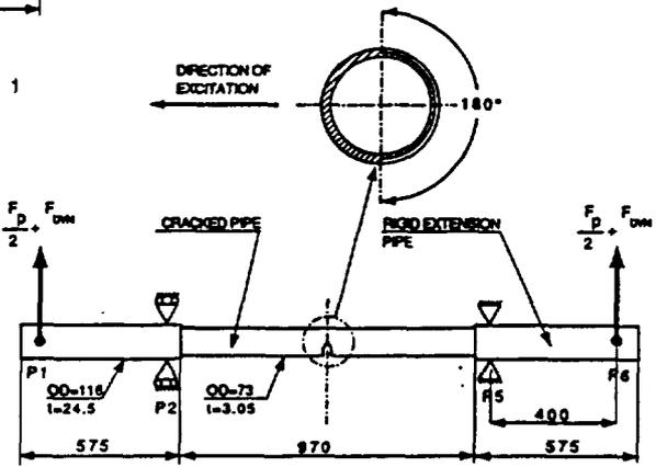
**DIMENSIONS OF CRACKED PIPE - Figure 2**
