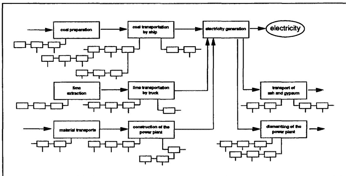
Fig. 2. Process analysis of a coal fired energy supply system.
