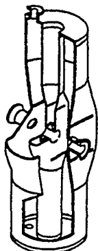
Fig. 2. A two-gap superconducting niobium resonator which was constructed and tested at ANL by Delaven, et al. [14].
