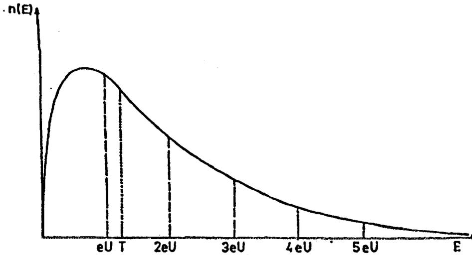
Figure 3. Boltzman energy distribution for the ions with temperature  $T$  and values of potential barrier for the charge states of  $i = 1 - 5$  [13].
