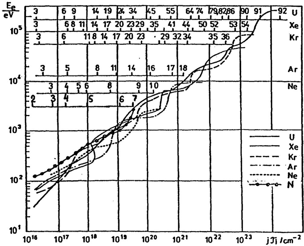
Figure 2. Calculated values of  $j\tau$ , required for producing Ne, Ar, Xe and U ions of a given charge state at corresponding energies of the electrons [2] added with the data for N.
