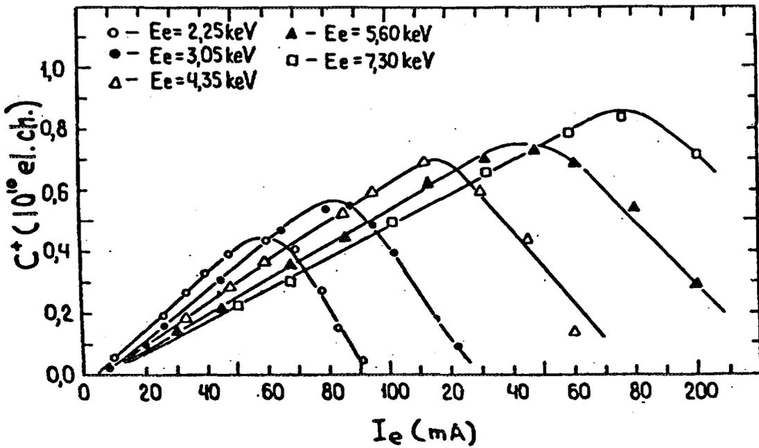
Figure 5. The dependence of the beam capacity on the beam current  $I$  for the different electron energies [2].
