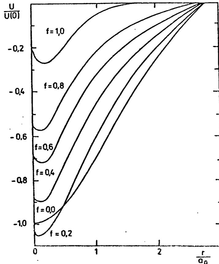
*Figure 1.* Dependence of the electrical field potential  $U$  on the beam radius  $r$  for various value of neutralization factor  $f$  [10].
