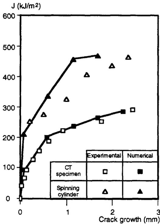
Figure 1 : Comparison of J-resistance curves derived from first spinning cylinder and CT-specimen tests.
