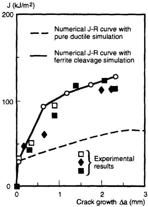
Figure 6 : Comparison of experimental and numerical J-resistance curves of aged duplex stainless steel.
