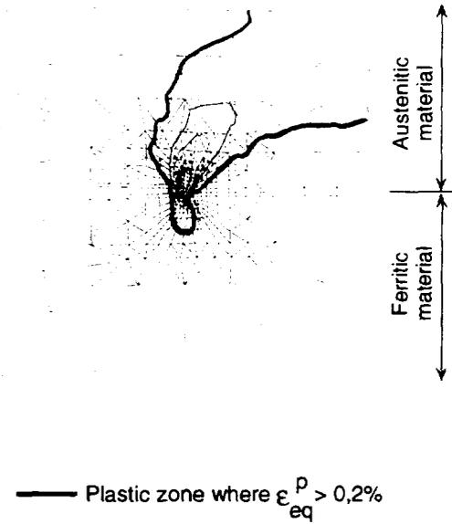
Figure 7 : Plastic zone extension at crack tip in a bimetallic CT specimen.
