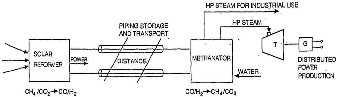
Fig. 7 Solar thermochemical concept reference system
