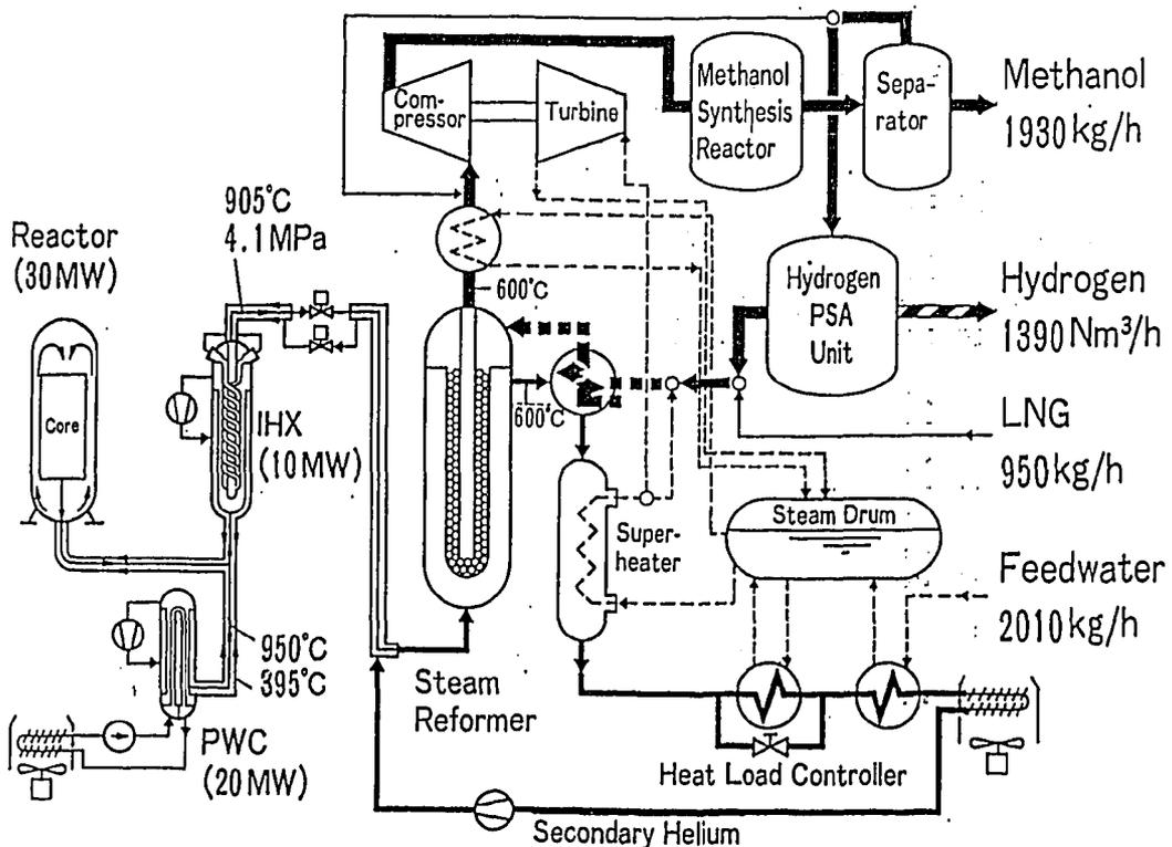
Fig. 5 Schematic Illustration of HTTR steam reforming hydrogen/methanol co-production system
