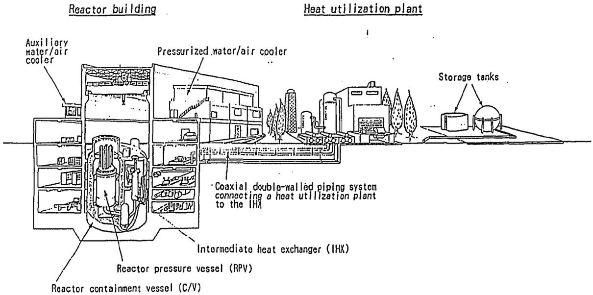
Fig. 2 Cutaway drawing of the HTTR plant with a heat utilization system
