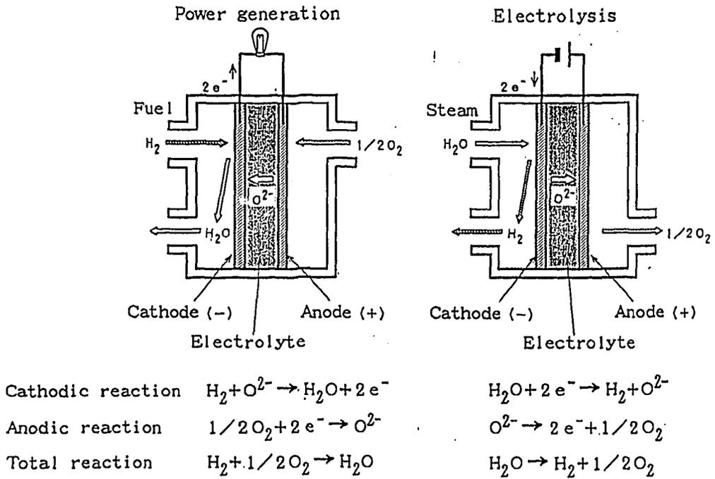
Fig. 8 Principle of high-temperature electrolysis of steam (Reverse reaction of solid oxide fuel cell)
