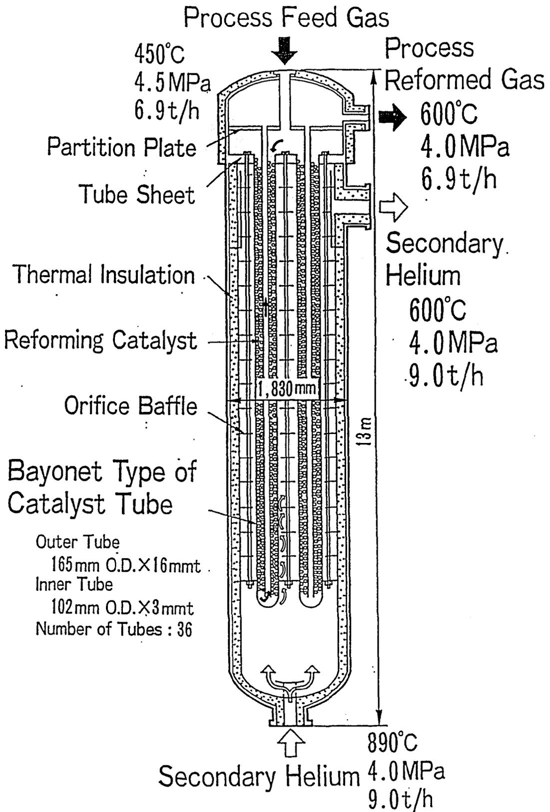
Fig. 6 Sectional view of steam reformer
