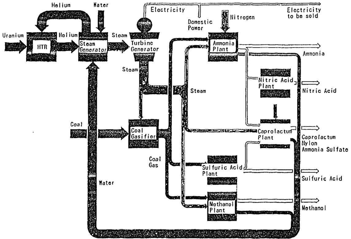
Fig.1 Diagram of HTR Co-Generation Plant
