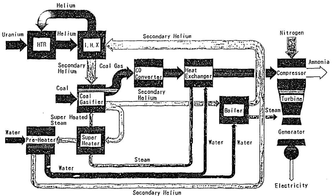
Fig.2 Diagram of HTR Coal-Gasification Ammonia Production Plant
