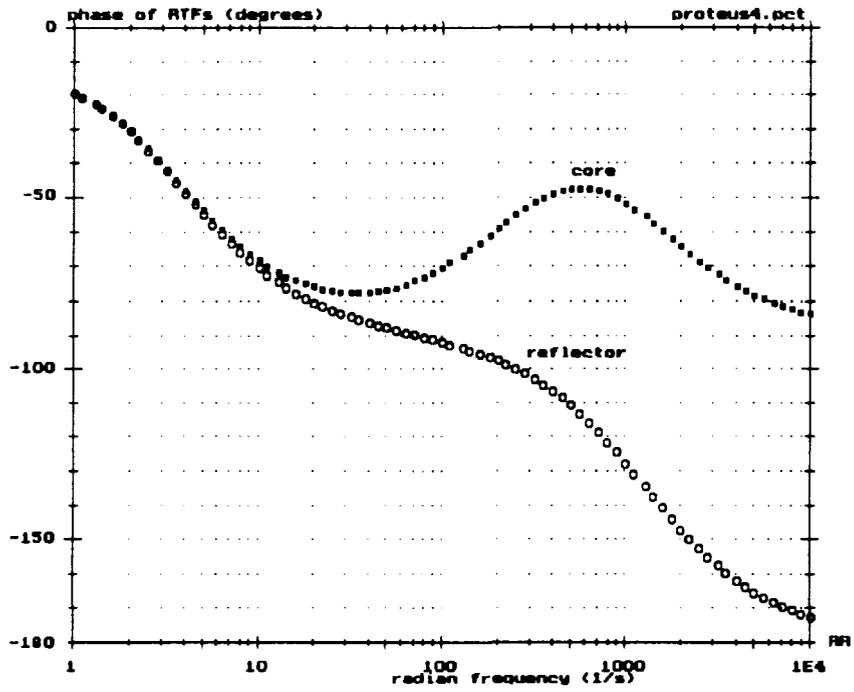
Figure 4. Phases of reactivity transfer functions of core and reflector for case 2.
