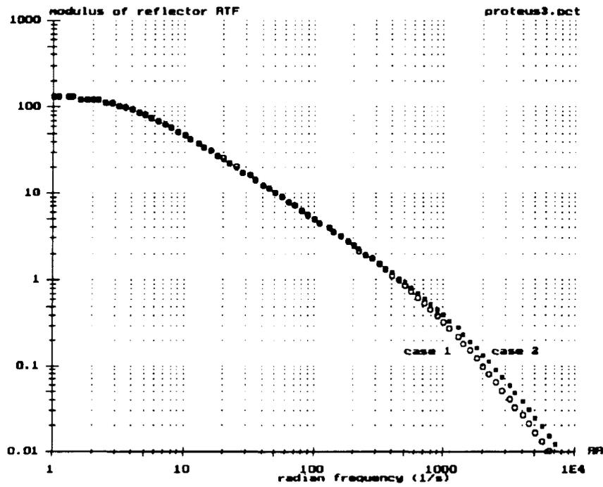
Figure 3. Moduli of reactivity transfer functions of the reflector.
