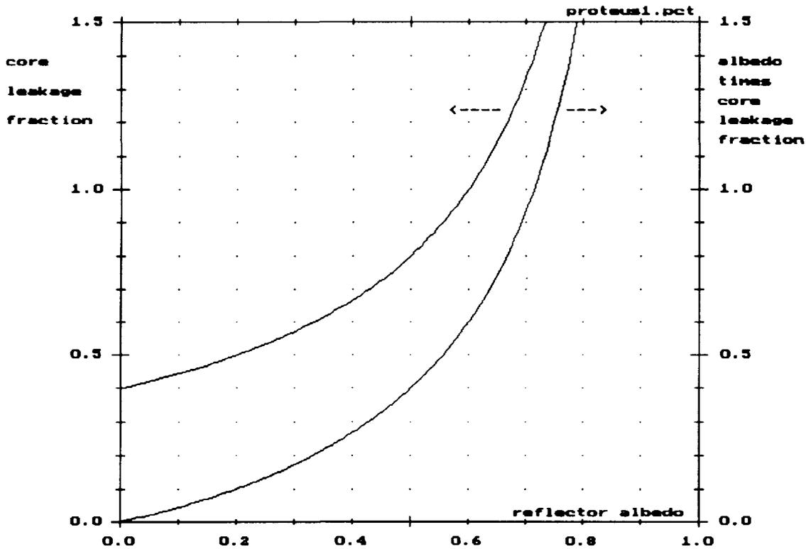
*Figure 1. Core leakage fraction and product of core leakage fraction and reflector albedo as a function of the reflector albedo for a critical PROTEUS-reactor.*
