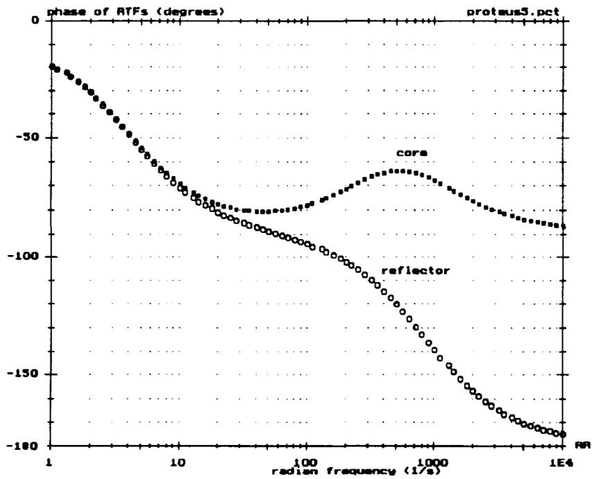
Figure 5. Phases of reactivity transfer functions of core and reflector for case 3.
