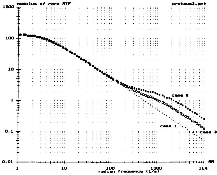
Figure 2. Moduli of reactivity transfer functions of the core.
