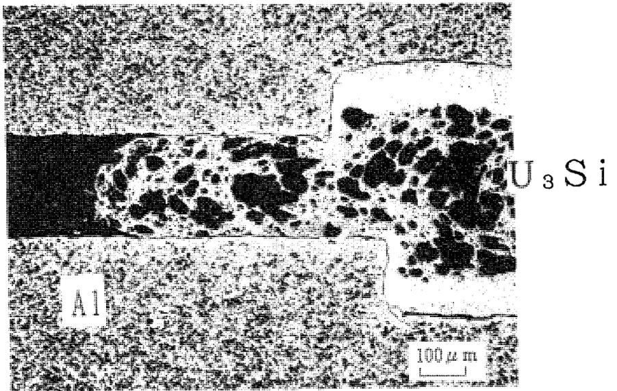
Fig. 6 Microstructure of  $U_3Si$  disk-type fuel, irradiated to 62 % at ~280 °C for 216 days
