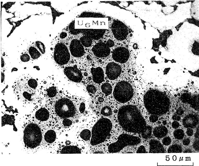
Fig. 5 Microstructure of Al-dispersion  $U_6Mn$  miniplate, irradiated to 53 % at 175 °C for 216 days
