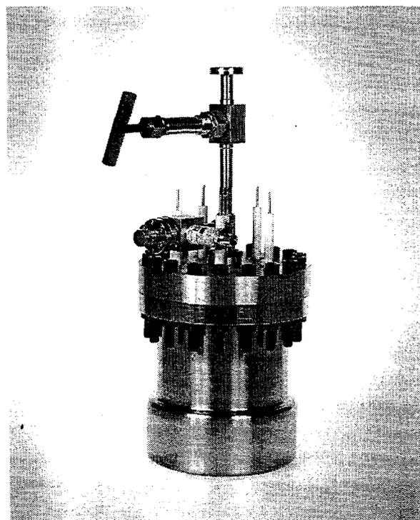
FIGURE 3. ASSEMBLED MARK II GAMMA-RAY SPECTROMETER
