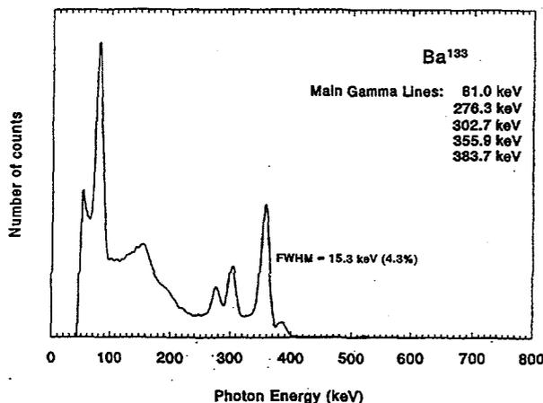
FIGURE 4. GAMMA-RAY SPECTRUM OF A  $^{133}\text{Ba}$  SOURCE
