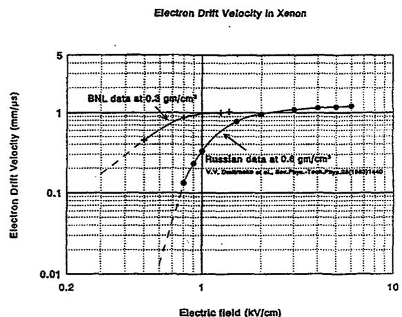
FIGURE 6. ELECTRON DRIFT VELOCITY IN XENON AS A FUNCTION OF APPLIED ELECTRIC FIELD
