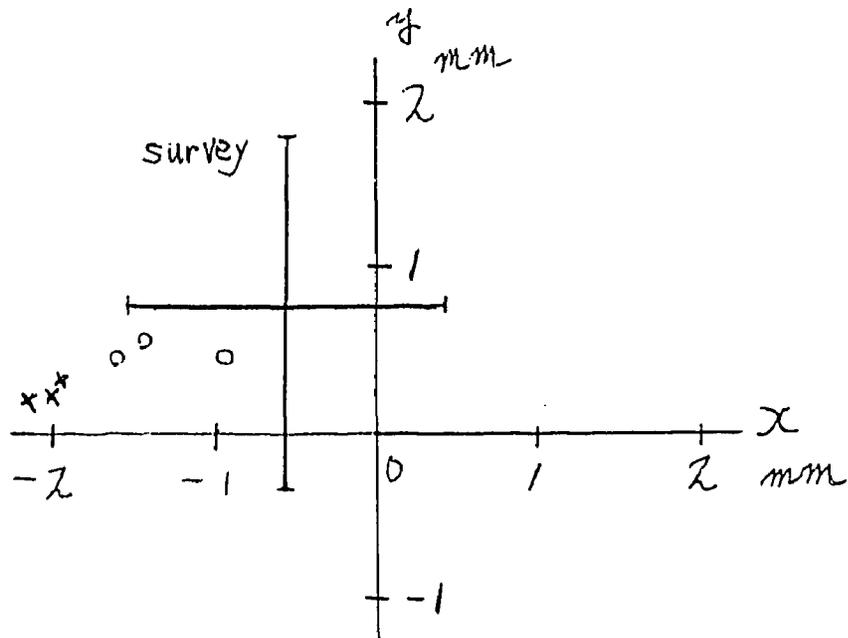
figure 1: Fitted x-y positions of the interaction point for tree run-periods. Circles show positions measured by the ESC and crosses by the CDC. The result of the optical survey is also shown.
