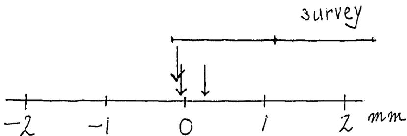
figure 2: Fitted z positions of the interaction point for tree run-periods by the ESC. The result of the optical survey is also shown.
