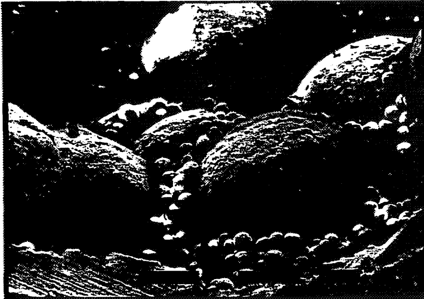
Figure 8.3 SEM picture of the top end of capsule 28.2 after unloading, showing resin impregnated pebbles: large beryllium pebbles and the mixture of small lithium-orthosilicate and small beryllium pebbles
