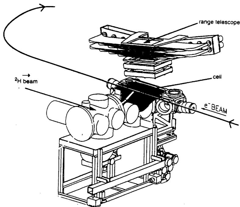
Fig. 6 - The AmPS polarized internal target facility.
