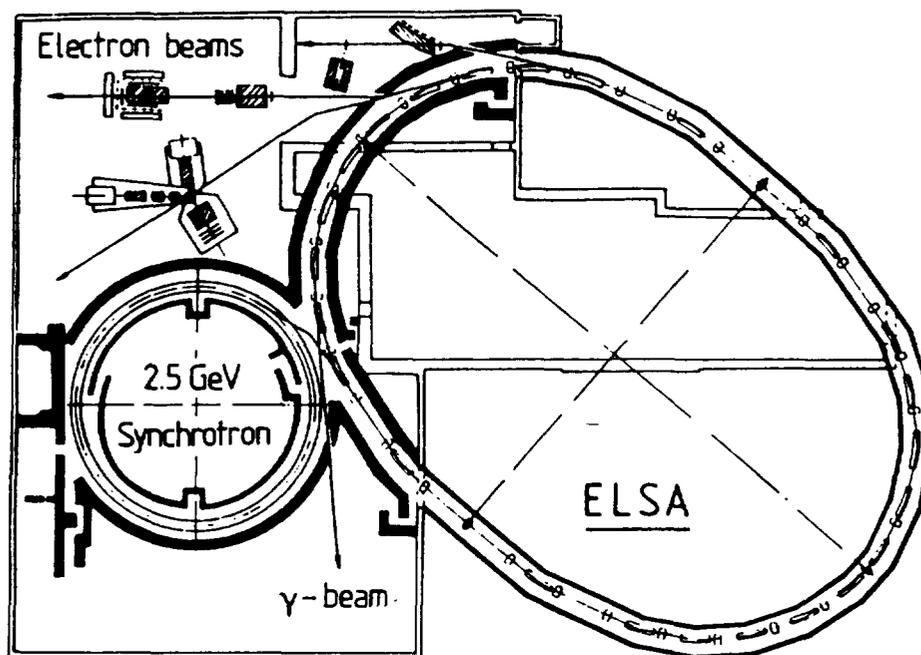
Fig. 7 - Plan view of the ELSA Synchrotron and Pulse-Stretcher Ring.
