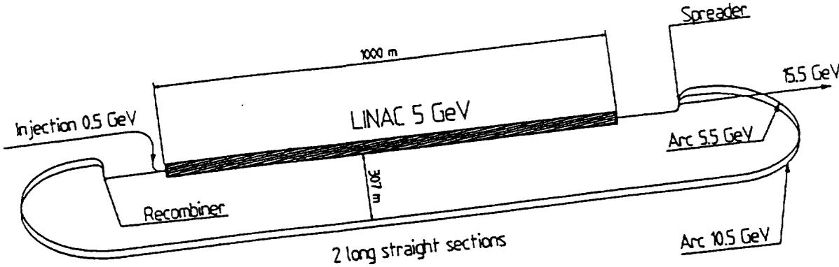
Fig. 10 - The ELFE project : a three pass single linac race-track.
