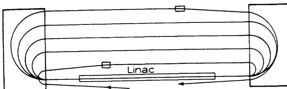
Fig. 1 - Scheme for a Race-track Microtron.
