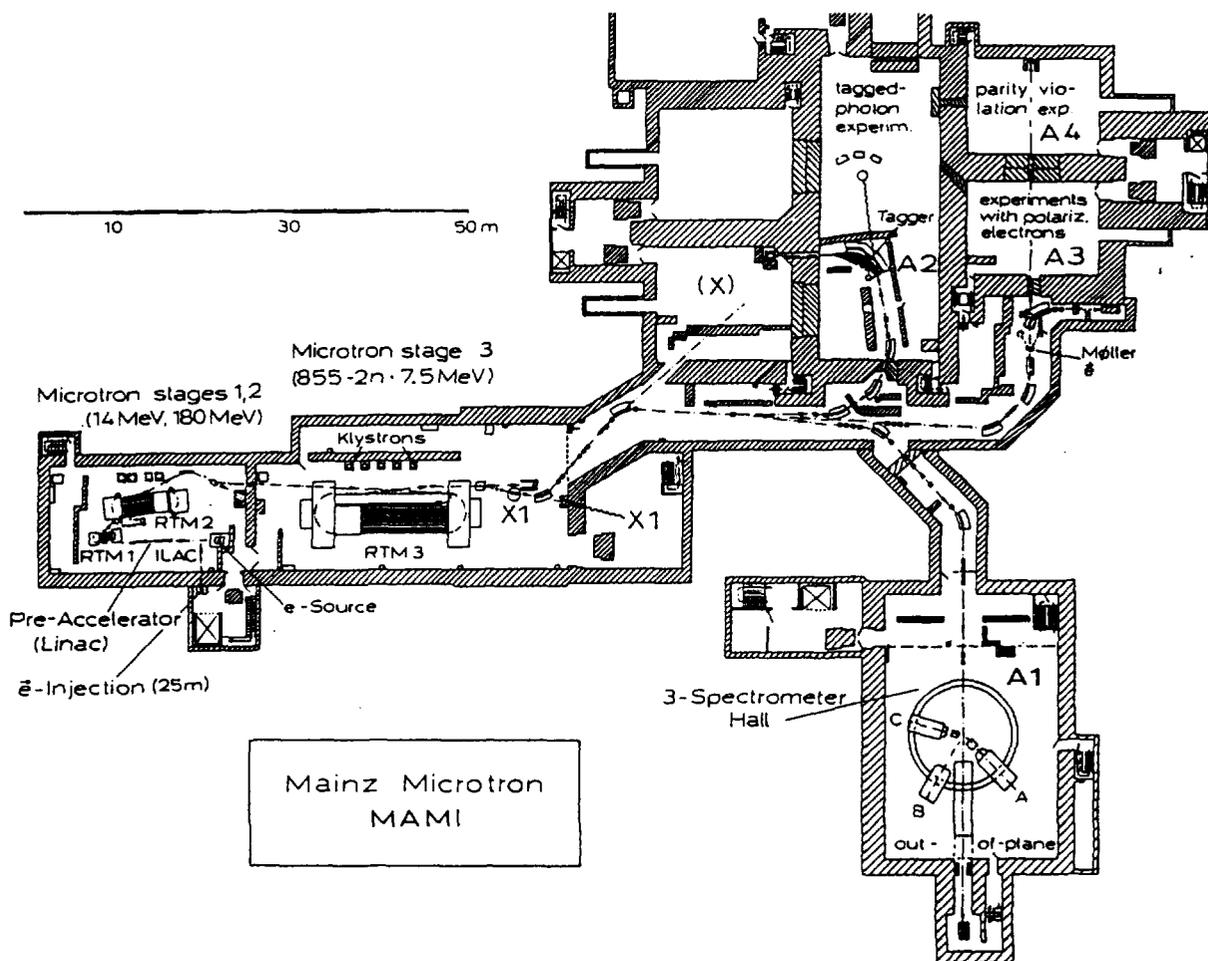
Fig. 3 - Floor Plan of the MAMI Microtrons and Experimental Areas.
