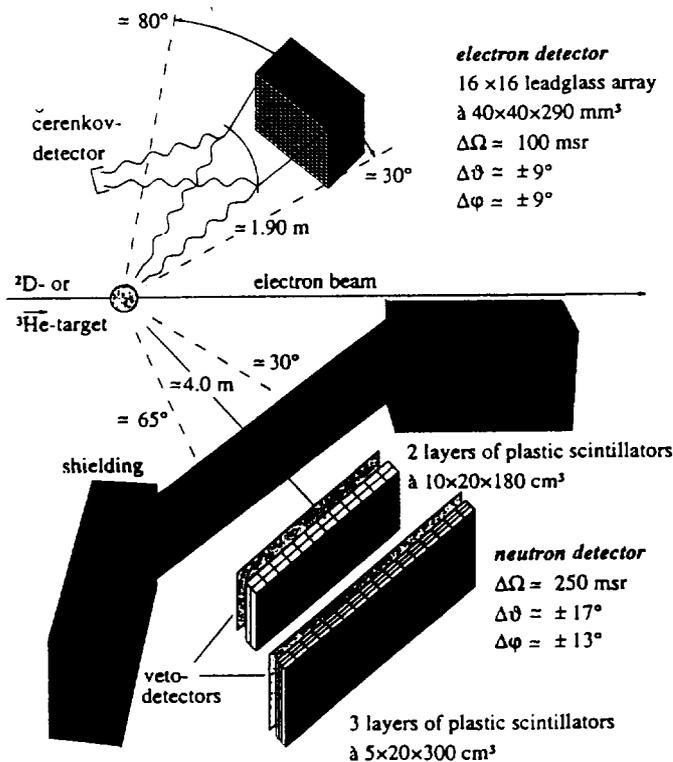
Fig. 4 - Set-up for the  $G_{E,n}$  experiments at MAMI.
