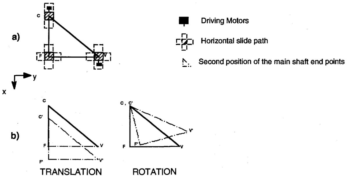
**Figure 2 Top view of the horizontal slides demonstrating translational and rotational motion when the motors are driven.**
