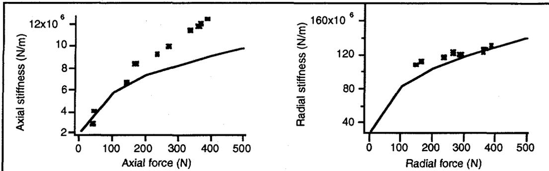
Figure 5 Comparison of experimental and theoretical results. (Markers show experimental results while continuous lines are used for theoretical results.)
