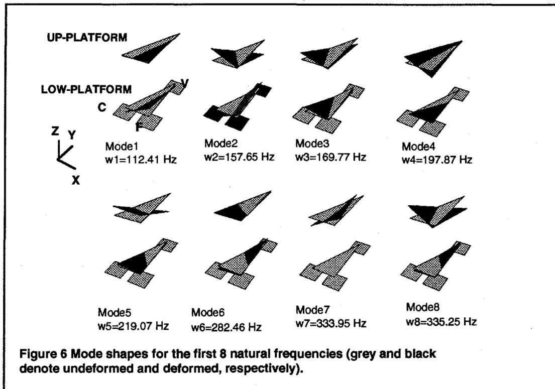
Figure 6 Mode shapes for the first 8 natural frequencies (grey and black denote undeformed and deformed, respectively).
