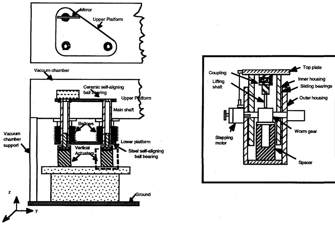
**Figure 1 Schematic of the mirror support system. (Detailed drawing of the vertical actuator is shown on the right)**
