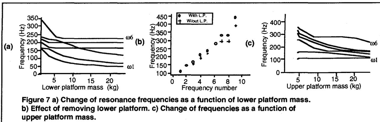
Figure 7 a) Change of resonance frequencies as a function of lower platform mass. b) Effect of removing lower platform. c) Change of frequencies as a function of upper platform mass.
