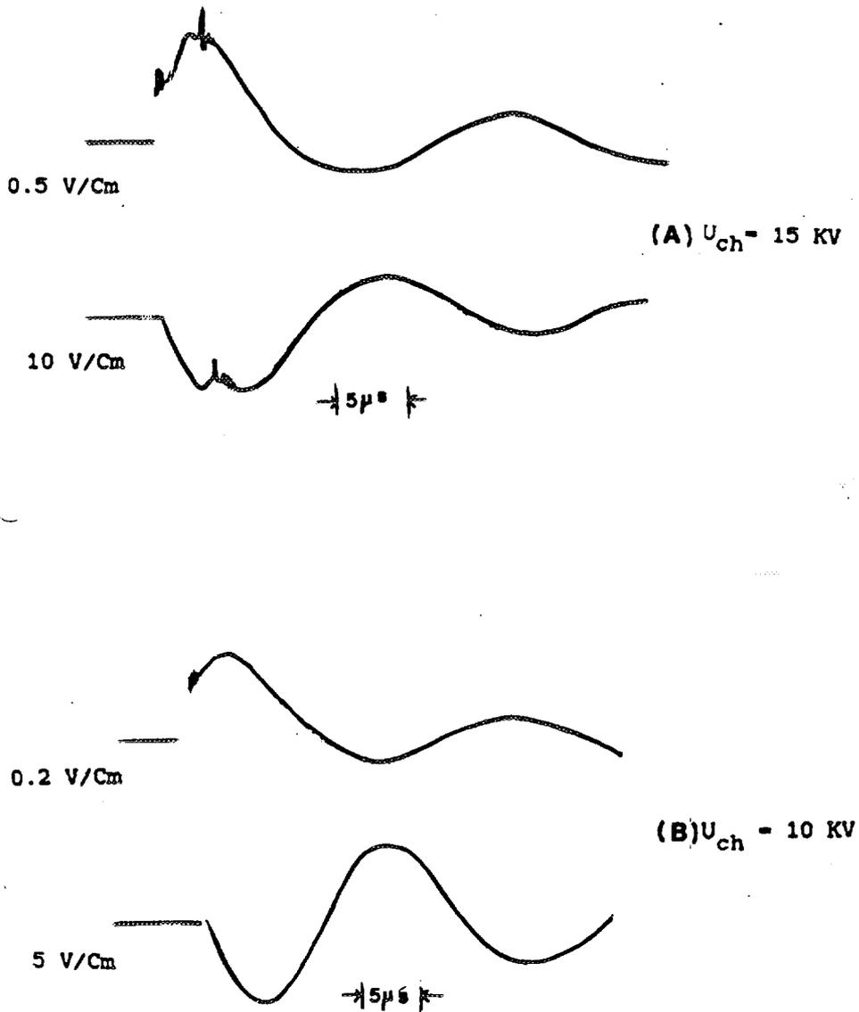
Fig.(7A,B): Oscillograms of breakdown voltage pulse (upper trace) and discharge current pulse (lower trace) for (A)  $U_{ch} = 15$  KV and for (B)  $U_{ch} = 10$  KV and  $P = 1.2 \times 10^{-1}$  Torr.
