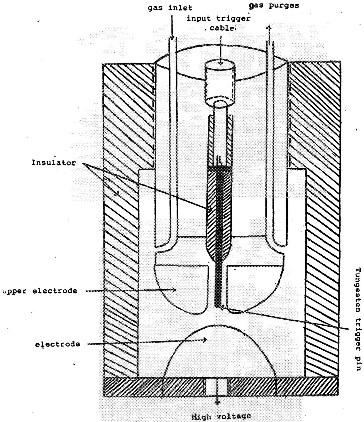
Fig. (3) : Pressurized spark gap switch.
