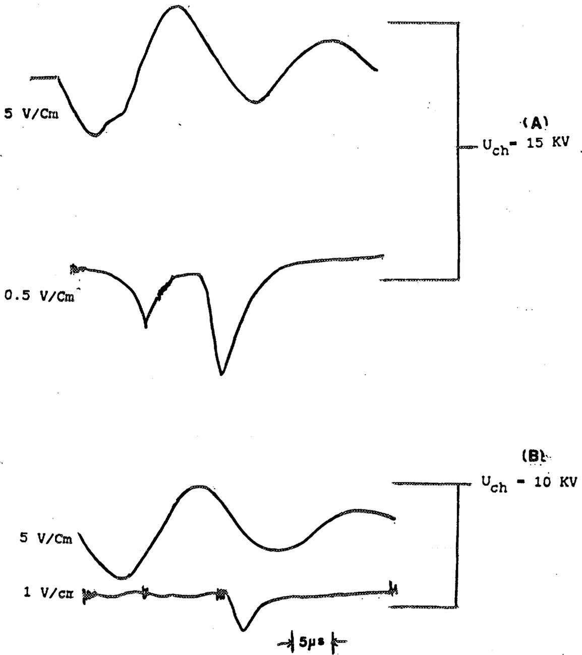
Fig.(9): Oscillograms of discharge current pulse (upper trace) and time structure of x-ray pulse (lower trace), for (A)  $U_{ch} = 15 \text{ KV}$  and for (B)  $U_{ch} = 10 \text{ KV}$ .  $P = 1.3 \text{ Torr}$ .
