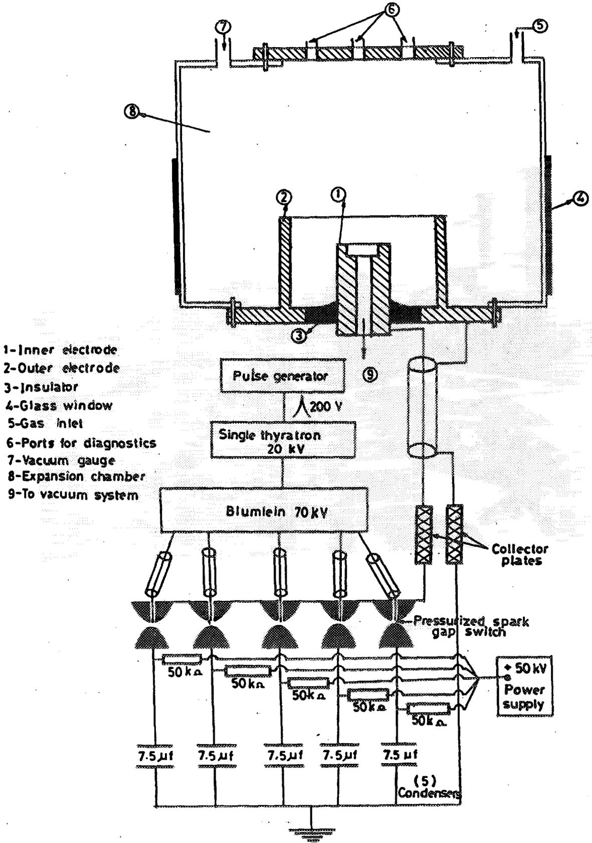
Fig.( 1 ): Cross section of the plasma focus apparatus.
