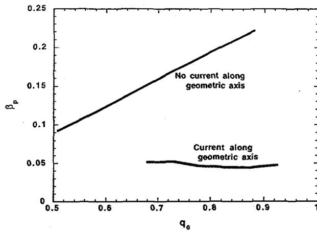
Fig. 3 Maximum Mercier-stable  $\beta_p$  as a function of  $q_0$  with and without current along the geometric axis.
