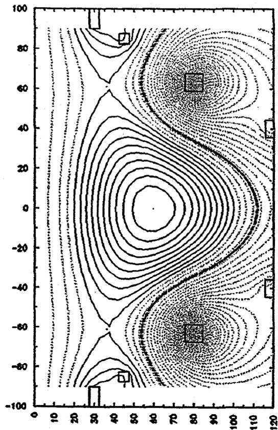
Fig. 2 Magnetic flux surfaces for the reactor design of Fig. 1.
