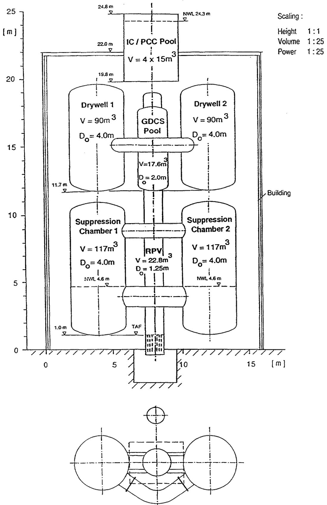
Figure 3 PANDA Experimental Arrangement
