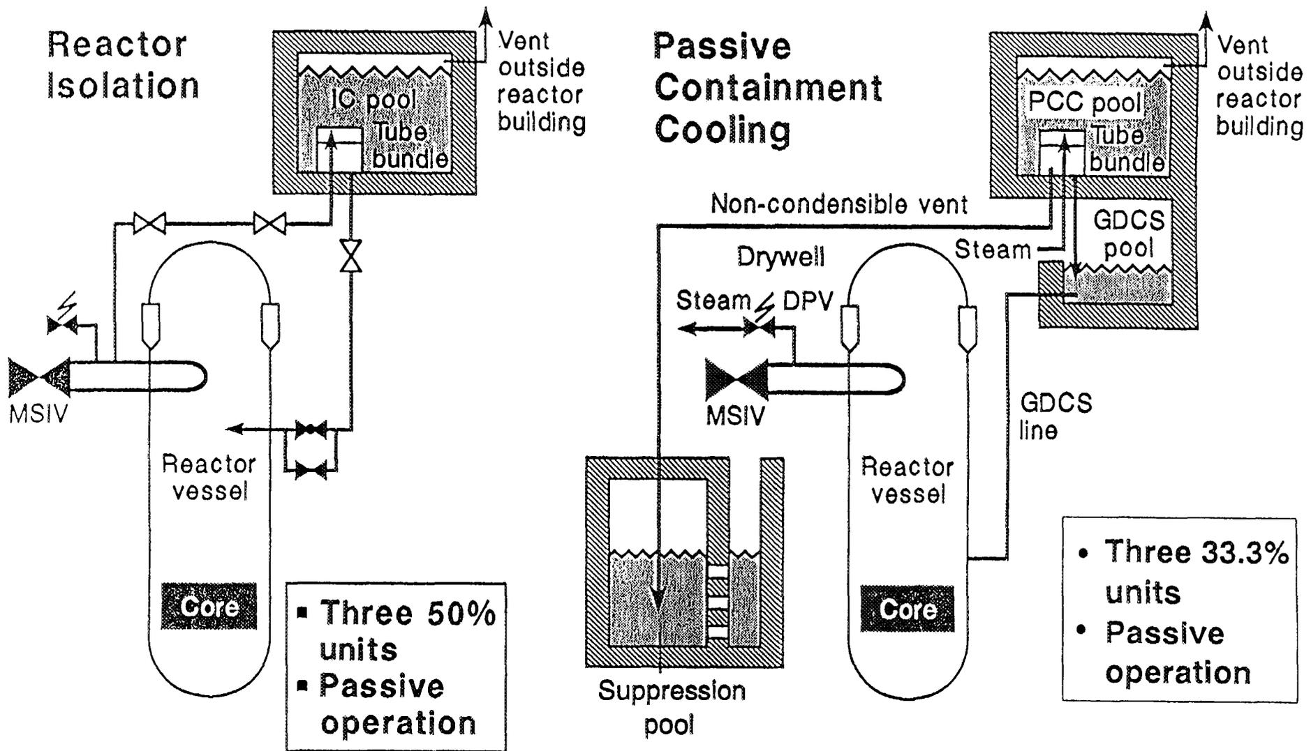
Figure 1 SBWR Isolation Condensers and Passive Containment Coolers
