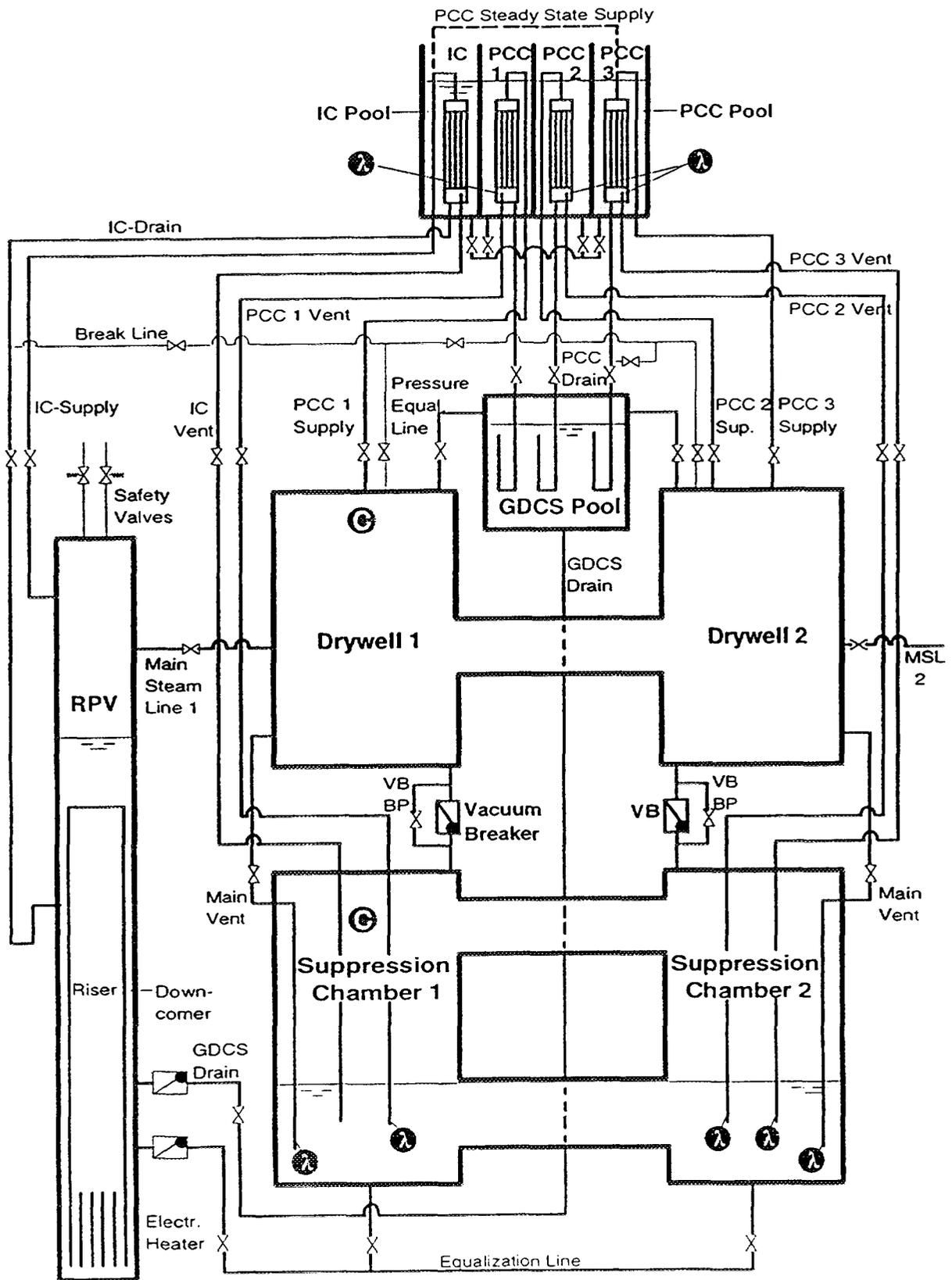
Figure 8 PANDA Instrumentation (Phase detectors and oxygen sensors)
