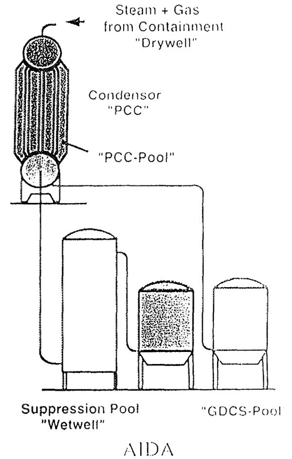
Figure 11 Schematic representation of SBWR and AIDA Test Rig
