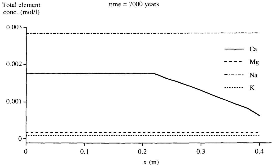
Figure 7.1.5 Total element concentrations of Ca, Mg, Na and K in the porewater of the bentonite buffer 7000 years after the sealing of the repository.
