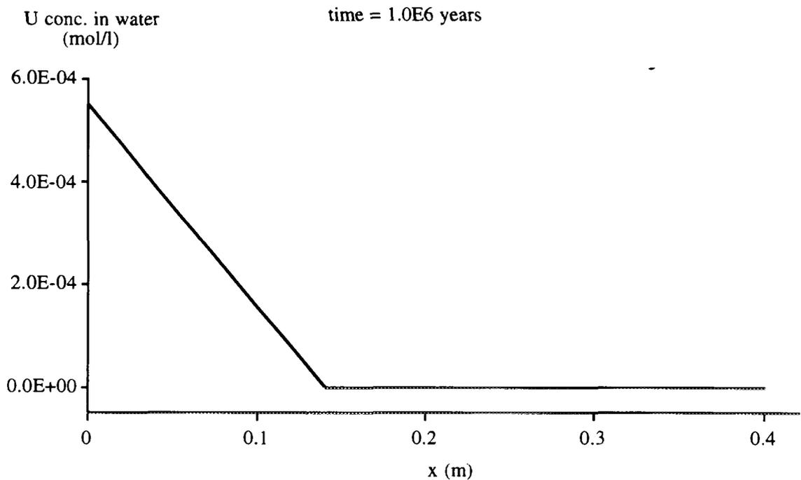
Figure 7.4.2 Profile of the total element concentration of uranium in the porewater in the bentonite buffer  $1.0 \cdot 10^6$  years after the sealing of the repository.
