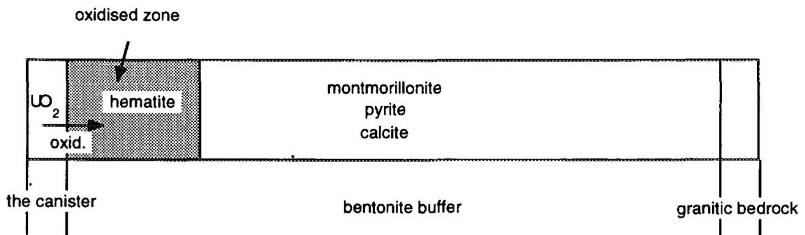
Figure 4.1 Model settings for the study of the stability of the bentonite buffer.
