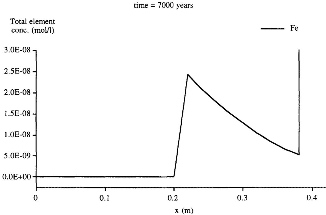
Figure 7.1.7 Total element concentrations of Fe in the porewater of the bentonite buffer 7000 years after the sealing of the repository.
