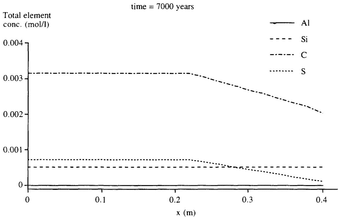
Figure 7.1.6 Total element concentrations of Al, Si, C and S in the porewater of the bentonite buffer 7000 years after the sealing of the repository.
