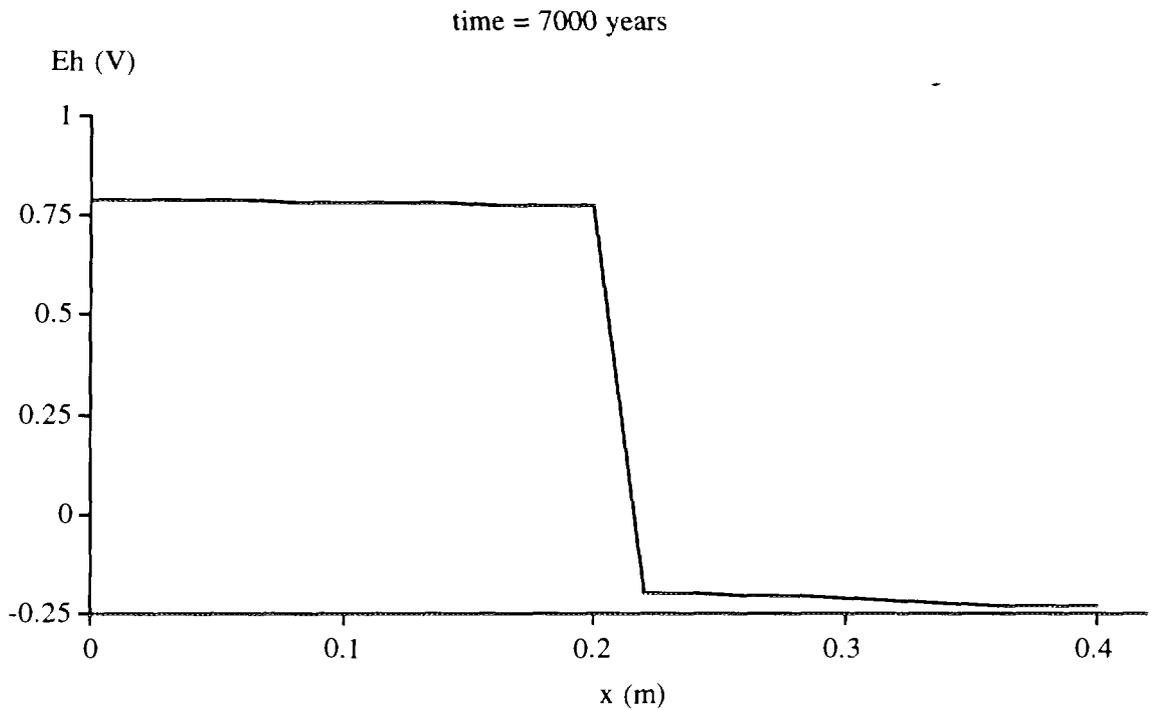
Figure 7.1.2 Eh (V) profile in the bentonite buffer 7000 years after the sealing of the repository.
