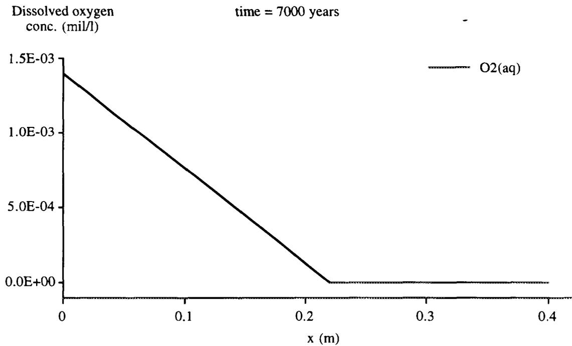
Figure 7.1.8 Dissolved oxygen concentration in the porewater of the bentonite buffer 7000 years after the sealing of the repository.
