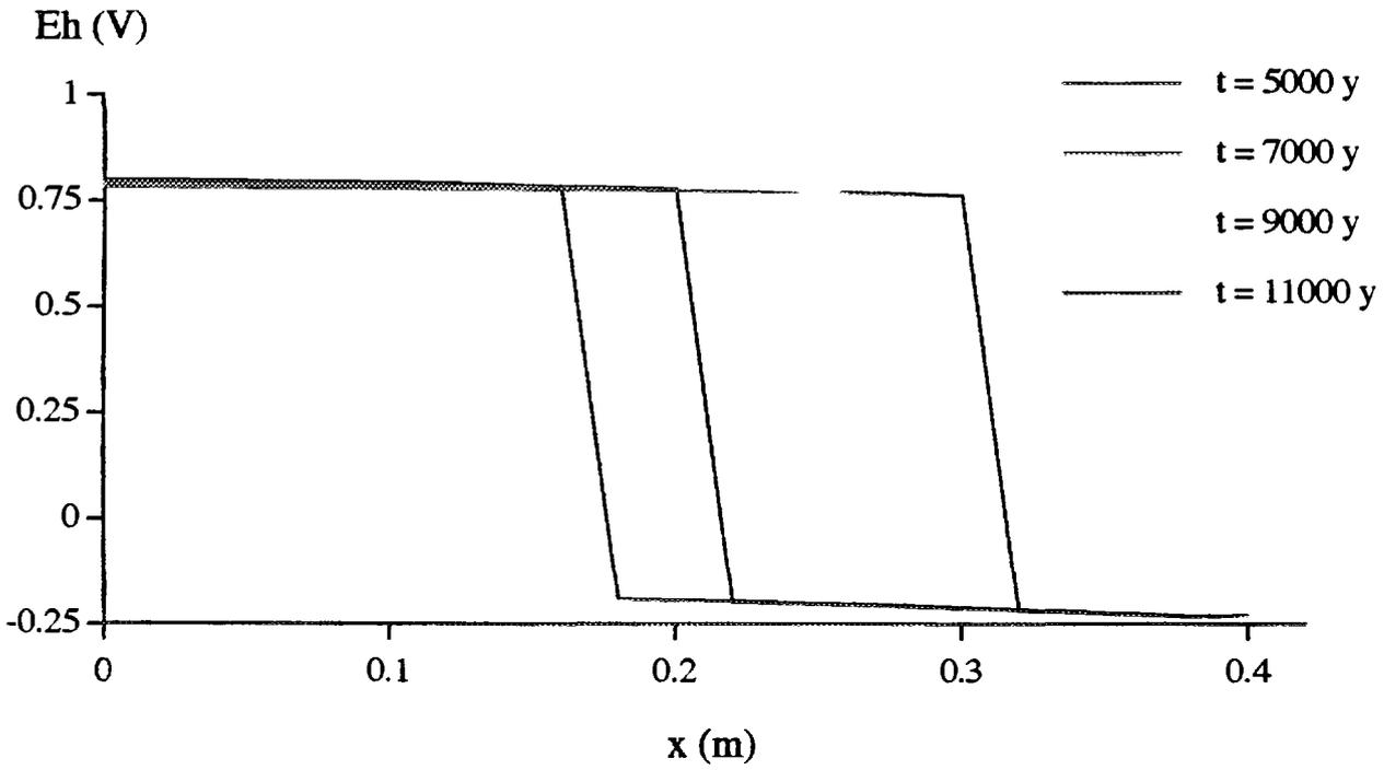
Figure 7.1.9 Changes of Eh (V) profiles in the bentonite buffer with time.
