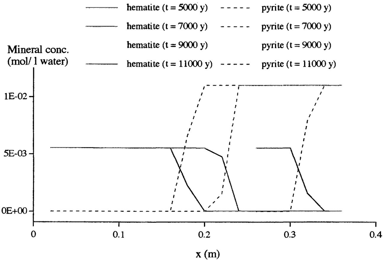
Figure 7.1.10 Changes of the contents of hematite and pyrite in the bentonite buffer with time.
