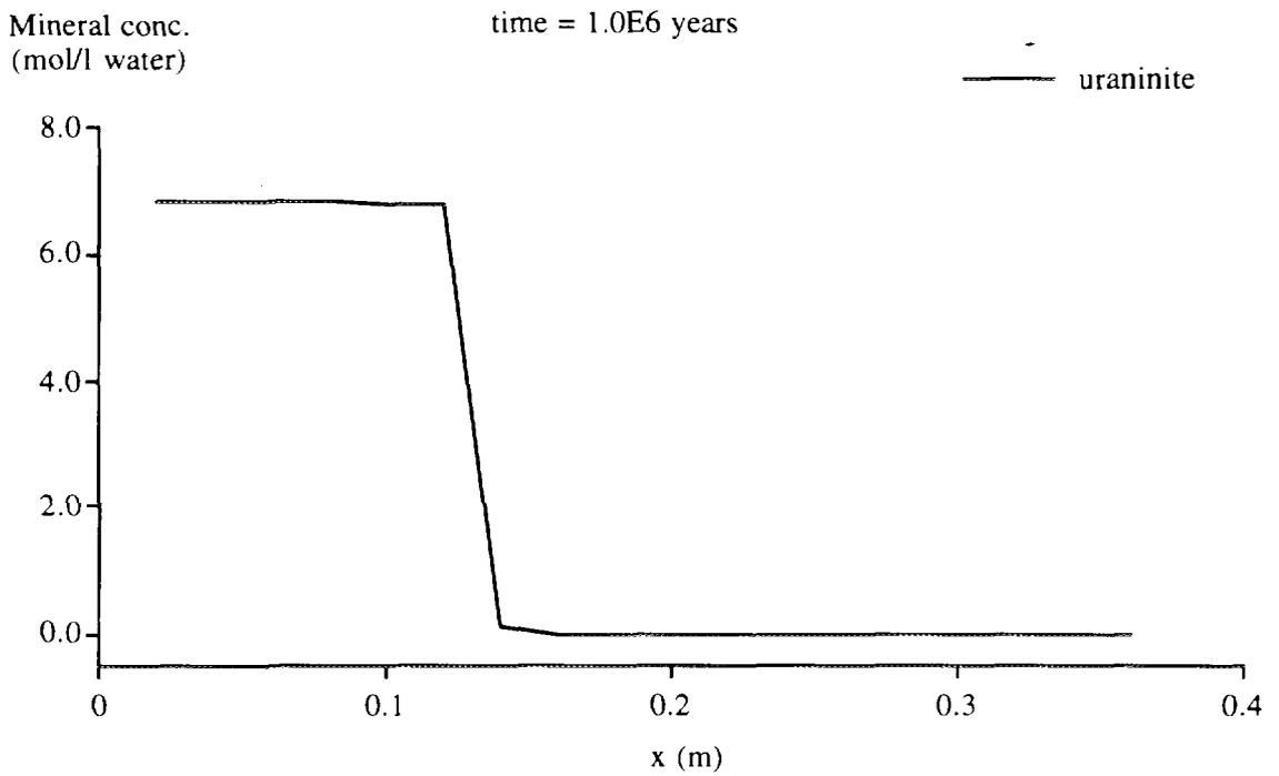
Figure 7.4.4 Concentration profile of uraninite in the bentonite buffer  $1.0 \cdot 10^6$  years after the sealing of the repository.
