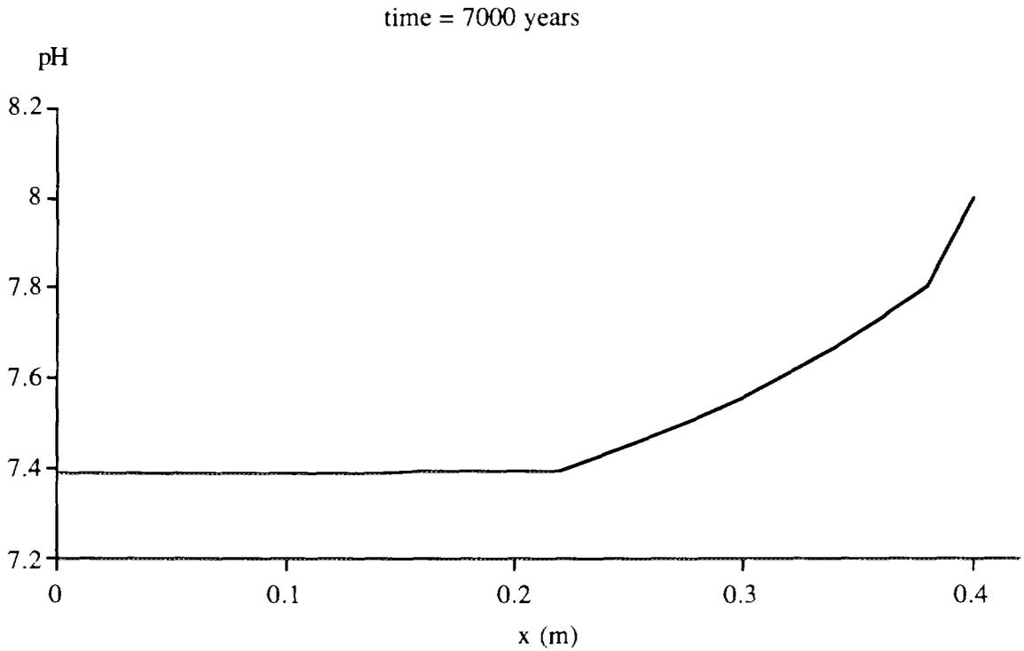
Figure 7.1.1 pH profile in the bentonite buffer 7000 years after the sealing of the repository.
