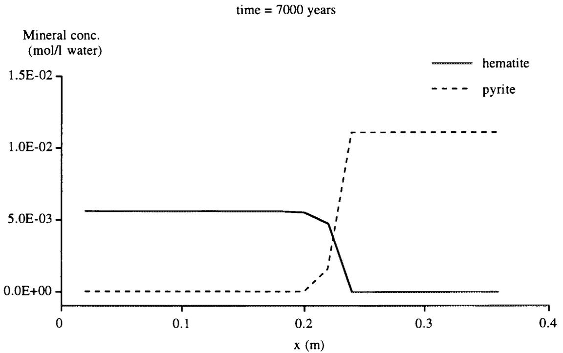
Figure 7.1.3 Contents of hematite and pyrite in the bentonite buffer 7000 years after the sealing of the repository. The vertical axis is in mol l<sup>-1</sup> of porewater.
