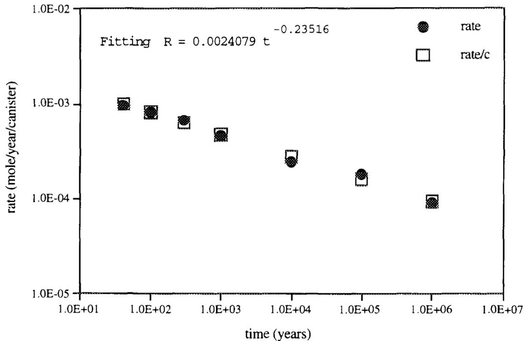
Figure 5.1 Data fitting for the rate of oxidant production by water radiolysis. The solid circles (●) are values from the literature (Christensen and Bjergbakke 1982). The squares (□) are values of data fitting. Both the rate and time coordinates are in logarithm scale.
