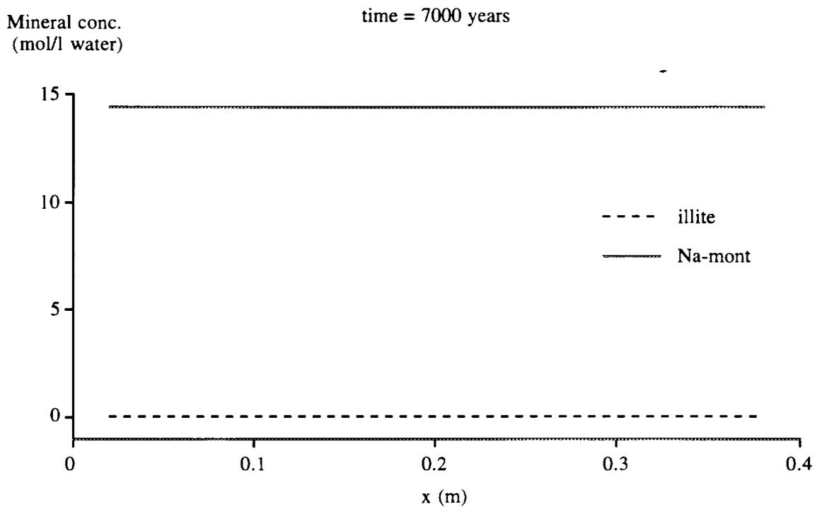
Figure 7.1.4 Contents of Na-montmorillonite and illite in the bentonite buffer 7000 years after the sealing of the repository. The vertical axis is in mol l<sup>-1</sup> of porewater. The content of illite is zero.
