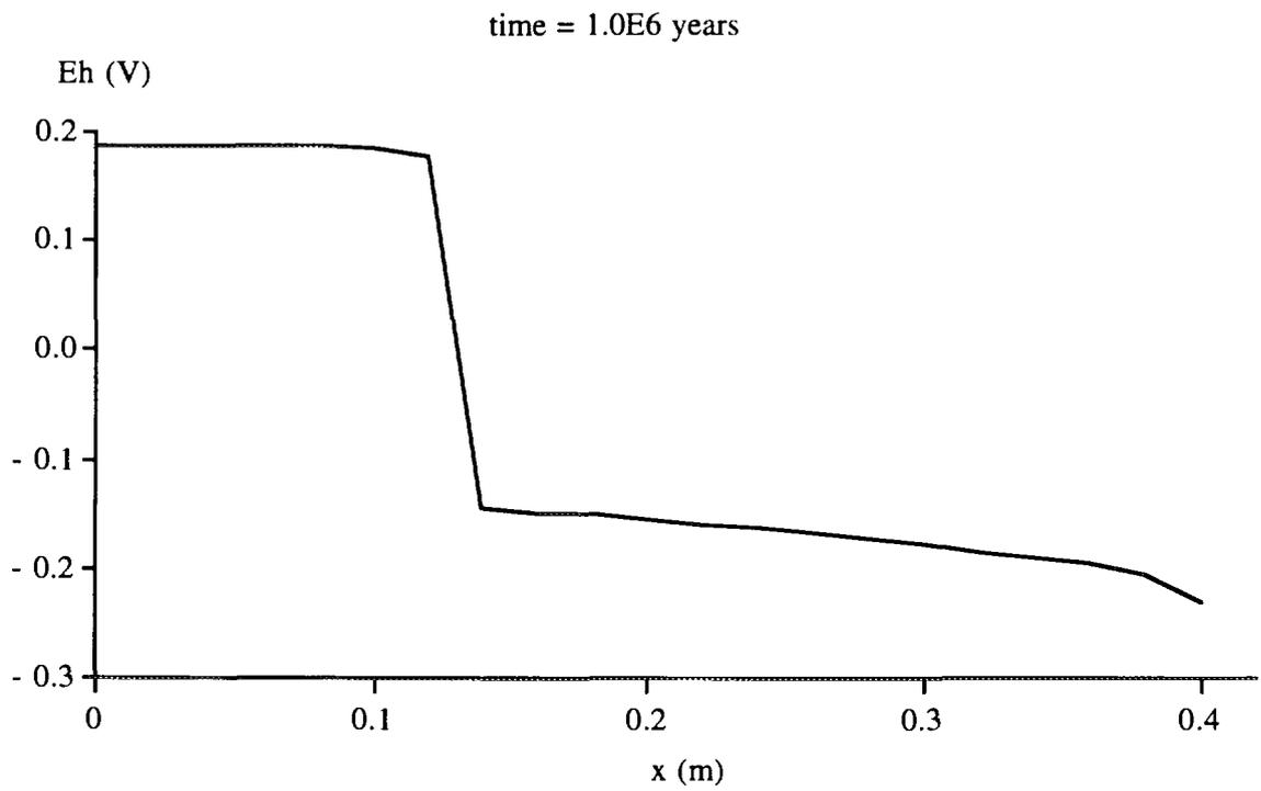
Figure 7.4.1 Eh profiles in the bentonite buffer  $1.0 \cdot 10^6$  years after the sealing of the repository.
