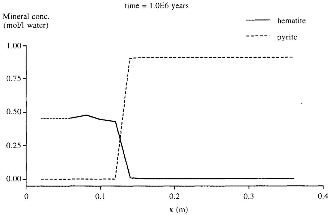
Figure 7.4.3 Concentration profiles of pyrite and hematite in the bentonite buffer  $1.0 \cdot 10^6$  years after the sealing of the repository.
