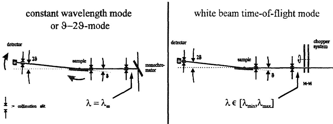
Fig. 1. Principal setup of a fixed wavelength and a white beam time-of-flight reflectometer
