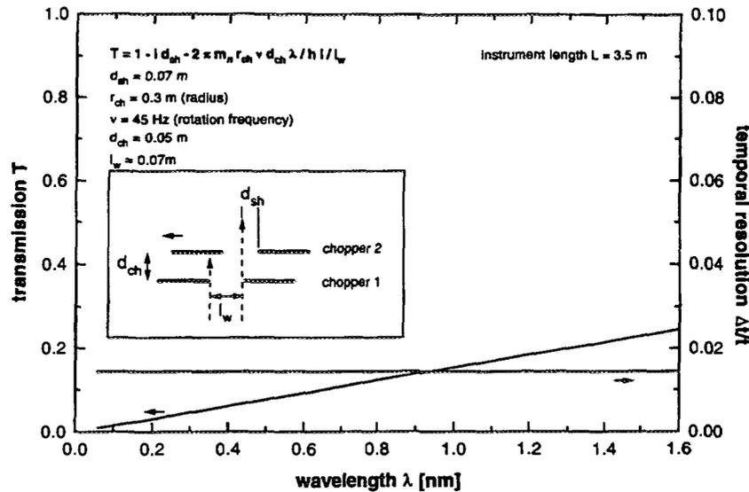
Fig. 6: Transmission function and temporal resolution, optimized for a  $\Delta t_{\text{pul}}/t = 0.014$  at a constant value
