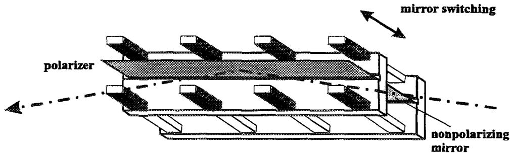
Fig. 7. Model for the principal arrangement of a polarizer and a second mirror in the deflecting unit
