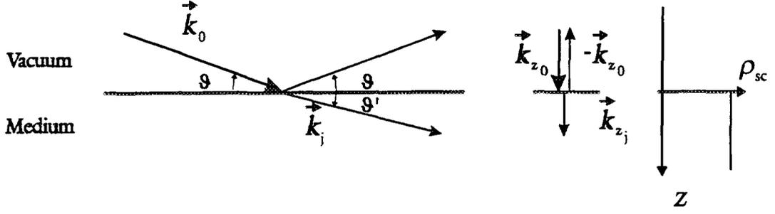
Fig. 2. Refraction of a wave at the interface to a medium  $j$ : geometry, normal components of the vectors, and scattering length density profile (from left to right)
