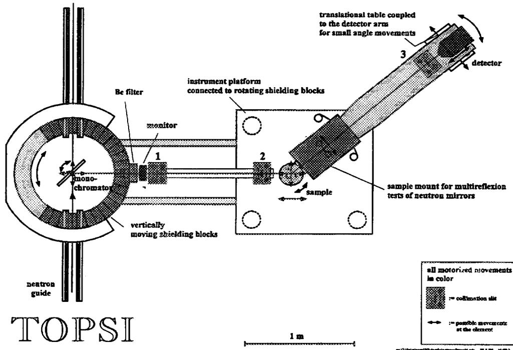
Fig. 3. Sketch of the TOPSI two axis spectrometer on a cold neutron guide
