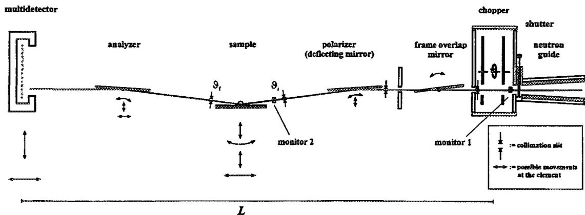
Fig. 5. Sketch of the overall instrumental layout of the proposed SINQ reflectometer. Components for the generation of magnetic fields and positioning aids are omitted.
