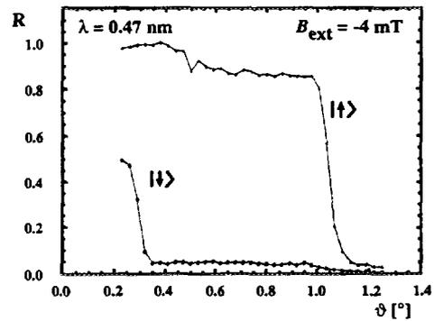
Fig. 9: Polarized neutron reflection from a 150 layer  $\text{Ti}_{1-u}\text{N}_u\text{-Fe}_{0.50}\text{Co}_{0.48}\text{V}_{0.02}$  supermirrors in the remanent state [28.].
