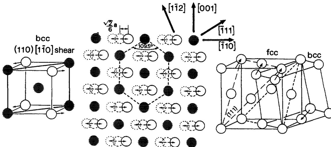
Fig. 12: Scheme of the bcc  $\rightarrow$  fcc transition.
